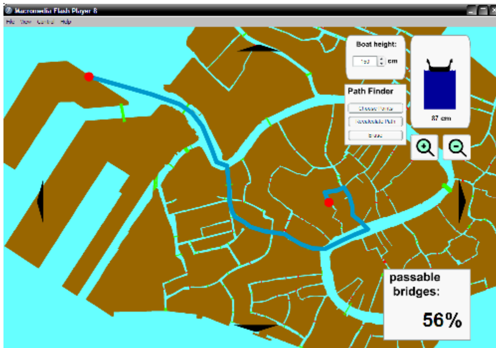
Figure 48: Another screenshot of the Acqua Alta Application, showing its planned future capabilities of mapping out the best routes based on tidal and boat information
