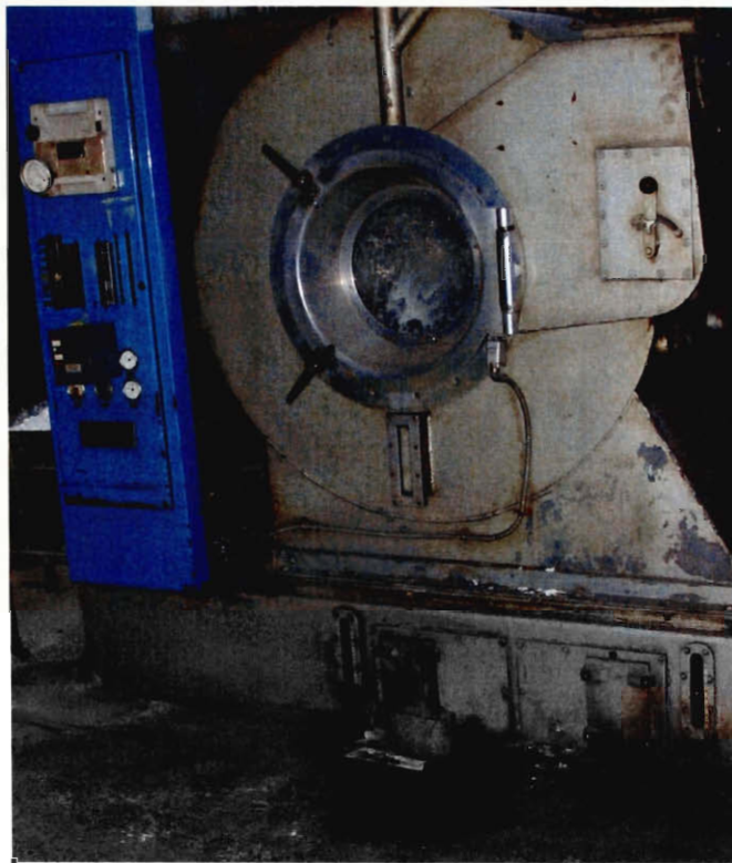
Figure 8: A Leaking First Generation Dry Cleaning Machine
