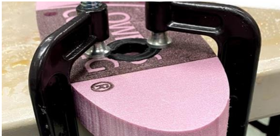
Figure 15: 3D printed part for the bottom of the trim tab housing drying after being glued.
