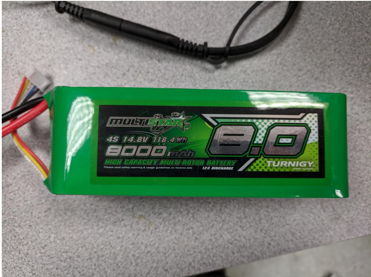
Figure 30: LiPo battery found in the lab and used for testing purposes.
