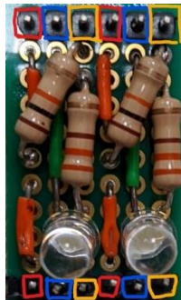
Figure 27: Practical implementation of the hall effect sensors. Red indicates 5V pins, blue indicated ground pins, and yellow indicates output pins. The two circuits are side by side and run top to bottom. The top is sensor side, and the bottom is microcontroller side.
