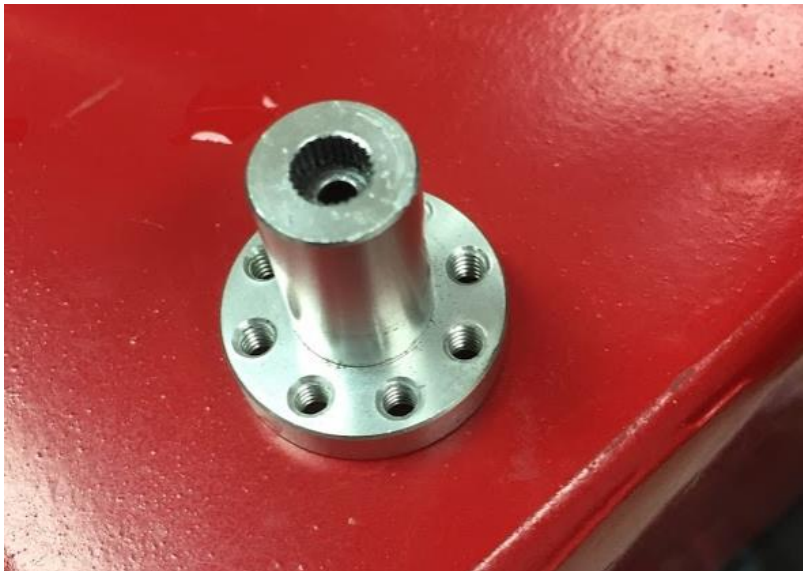
Figure 18: Stripped servo horn
