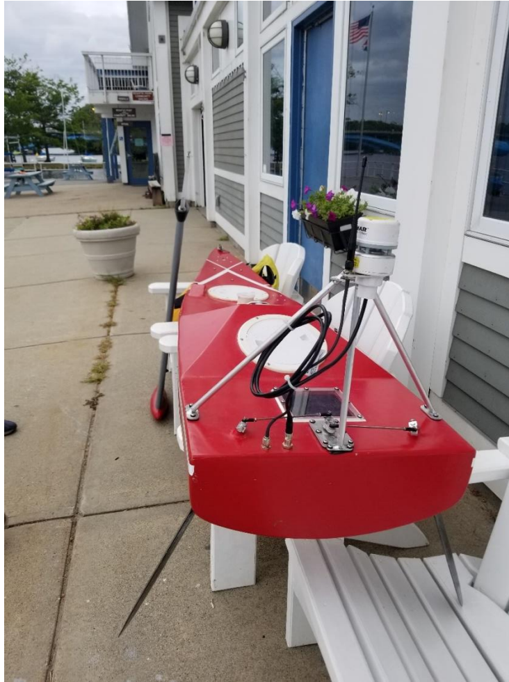
Figure 25: Boat with rudders and Airmar mounted. Note the lack of a winch provision in the hull.
