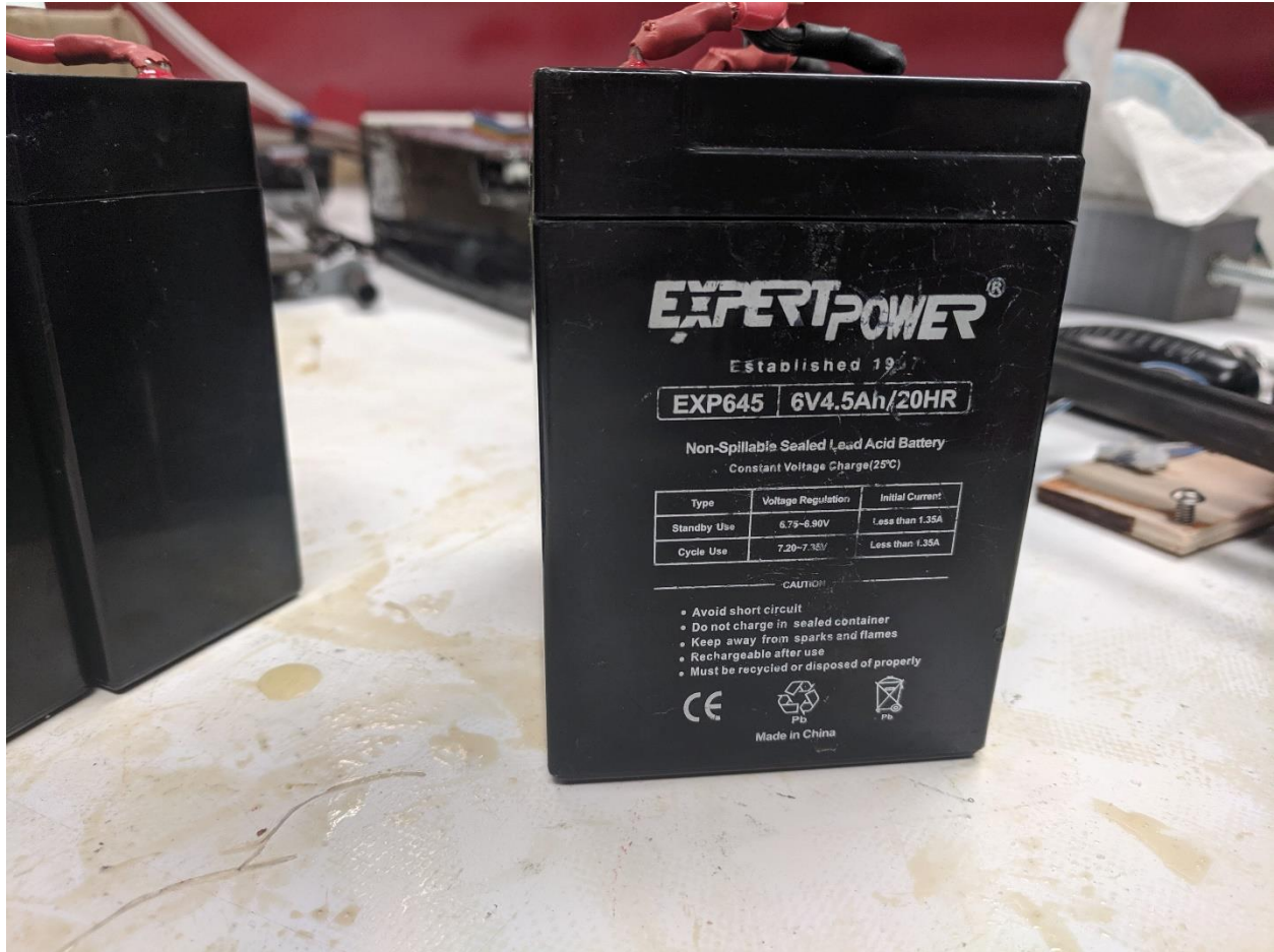
Figure 28: Lead-Acid battery used previously to power the system on the boat.
