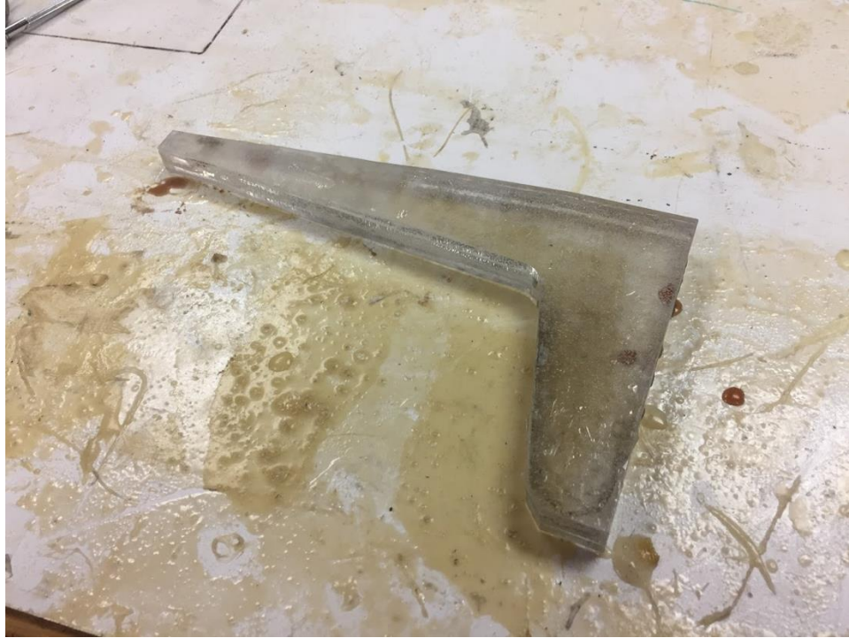
Figure 6: Polycarbonate insert for sealing the keel insert cavity
