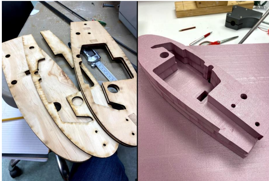
Figure 12: The existing foam cutting templates and the newly cut foam before further modifications.
