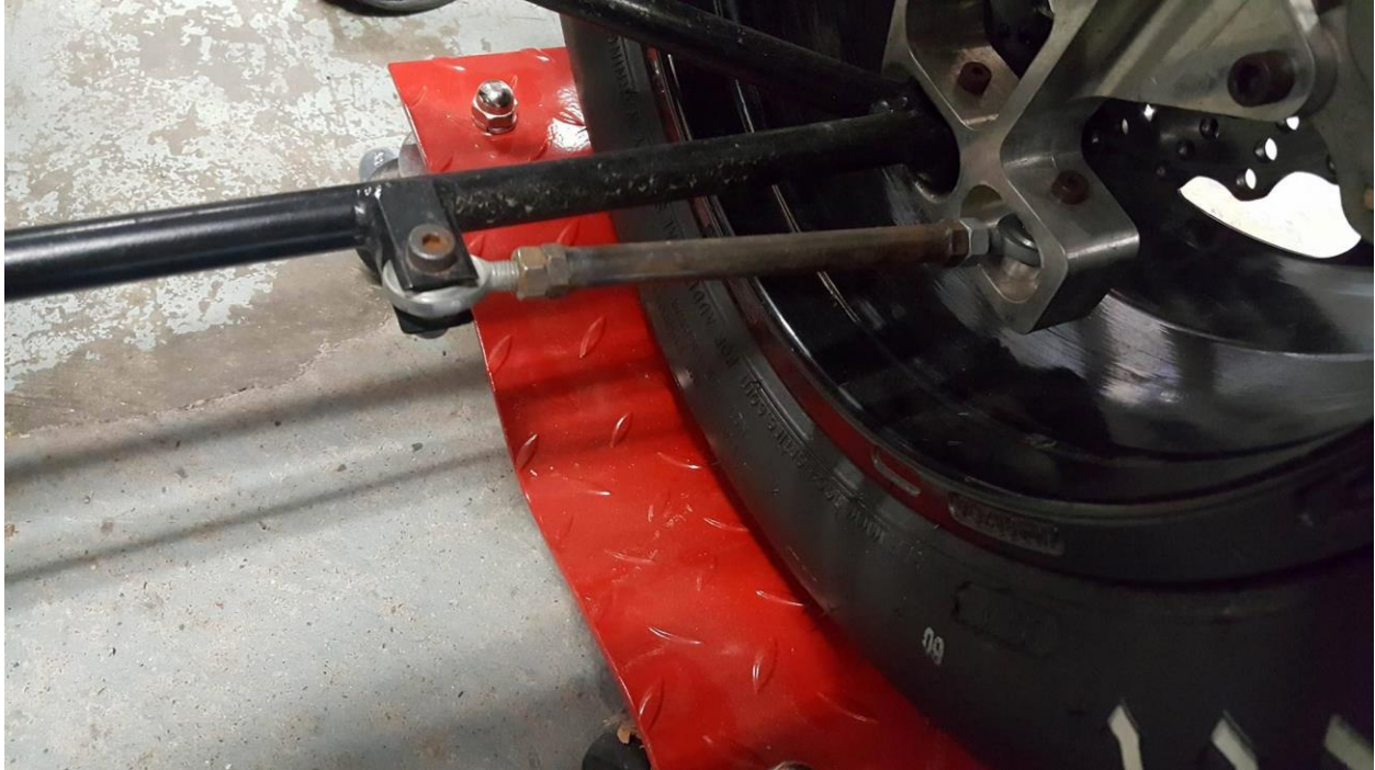
Figure 43: Previous toe bar design
