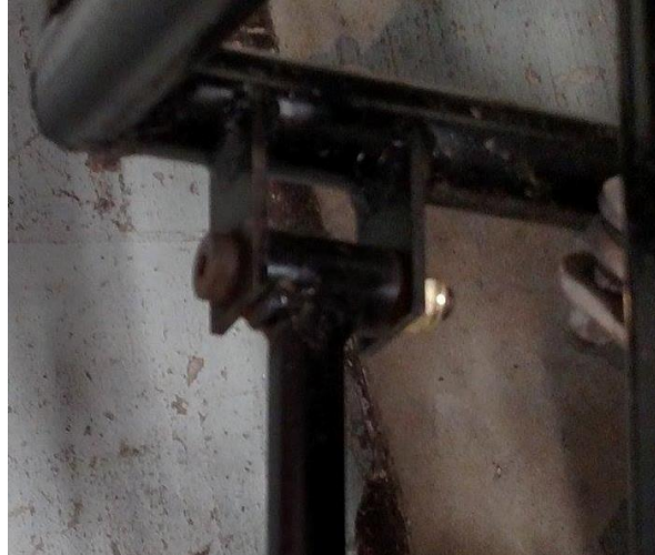
Figure 32: 2016 Single DOF suspension joint
