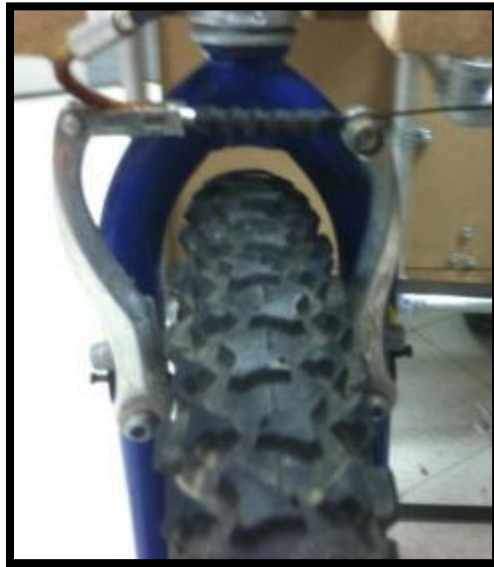
Figure 114: Parking V-Brake on Device Wheel
