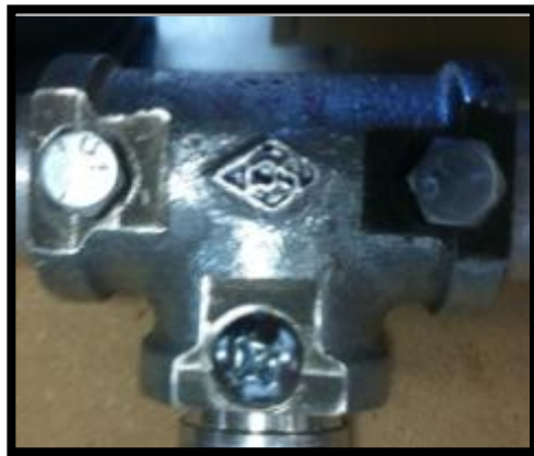
Figure 92: T fitting with three bolt fits
