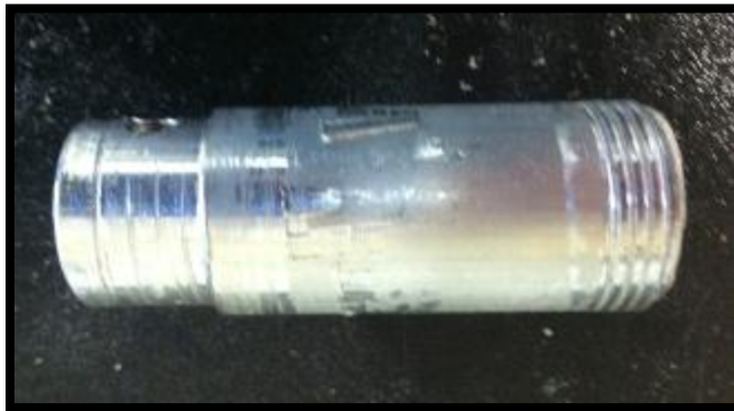
Figure 91: Piece of tubing that will be bolted on the left and threaded on the right
