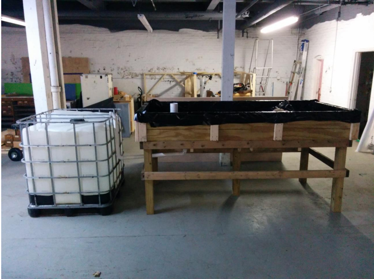
Figure 11. Constructed Prototype. Left: Fish Tank; Right: Bed & Stand. Piping has not been cemented yet.
