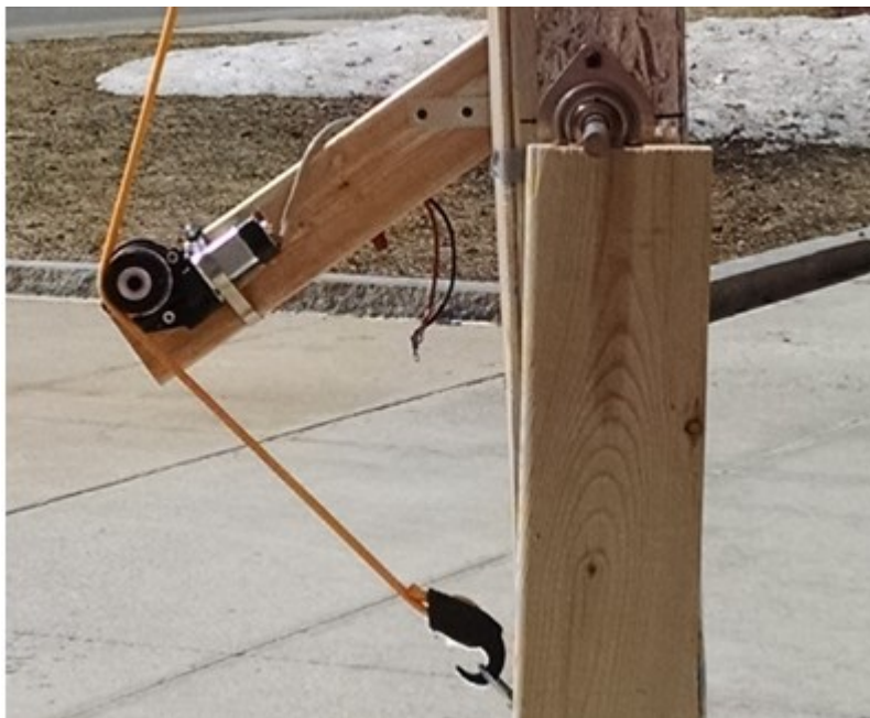
Figure 68 Mounted Electric Motor
