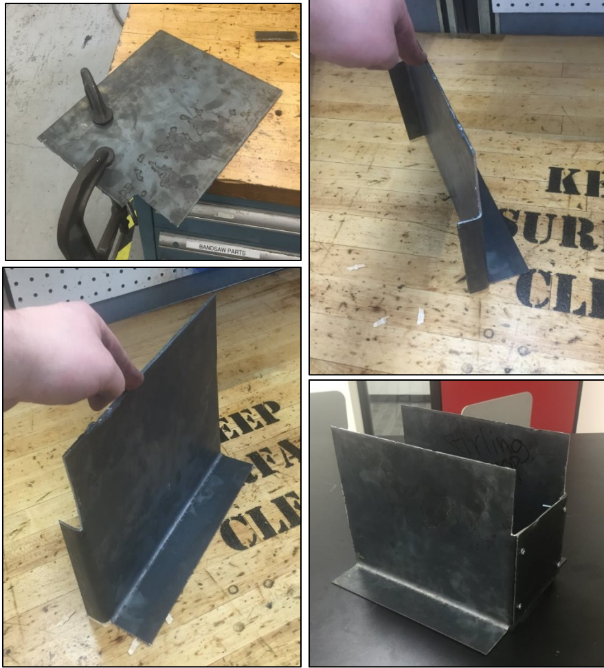
Figure 27 Engine Mount Fabrication
