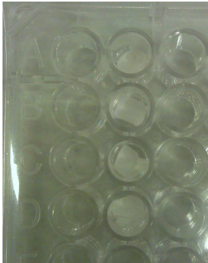
96 well plate containing 4 6 mm by 6 mm sheets of the electrospun scaffold after EtO gas sterilization.
