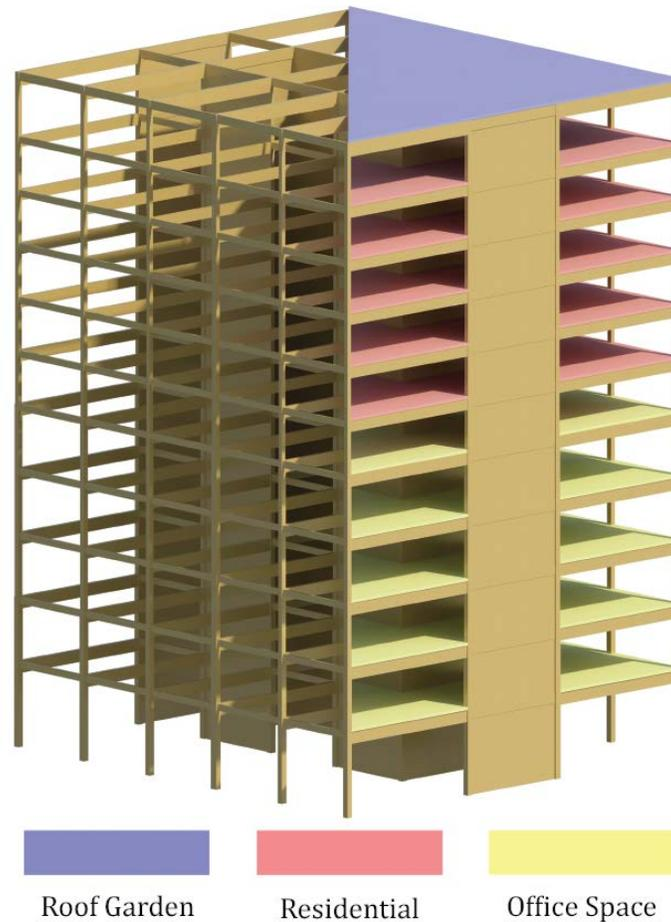
*Figure 5: Render of the mass timber frame with color coded loading conditions*
