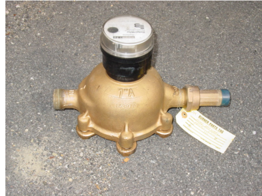
Figure 12: Water Meter and reader
