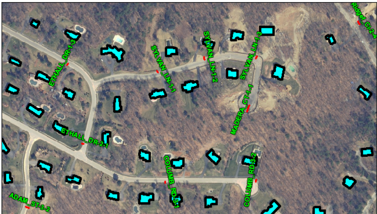
Figure 22: Hydrant Connections with ID Codes
