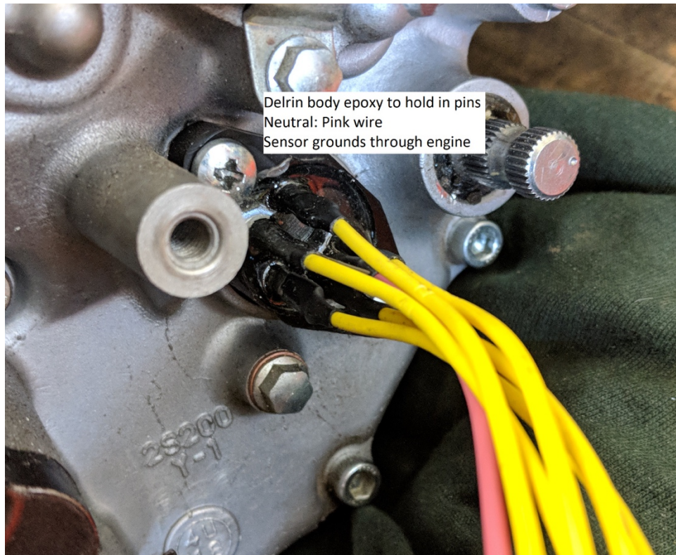
Figure 65: Gear indicator sensor installed
