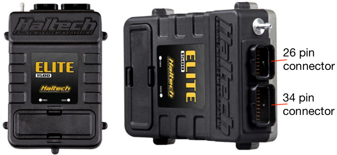
Figure 28: Haltech Elite 1500 ECU [23]. Two connectors are used: A 26-pin connector and a 34-pin connector. Various connections on each are used.
