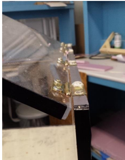
Figure 16: Hinge connection used in test section construction
