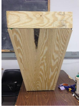
Figure 11: Completed contraction section, side view
