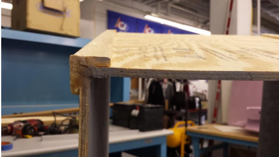
Figure 13: Wooden corner guard connecting plywood sides of diverging section
