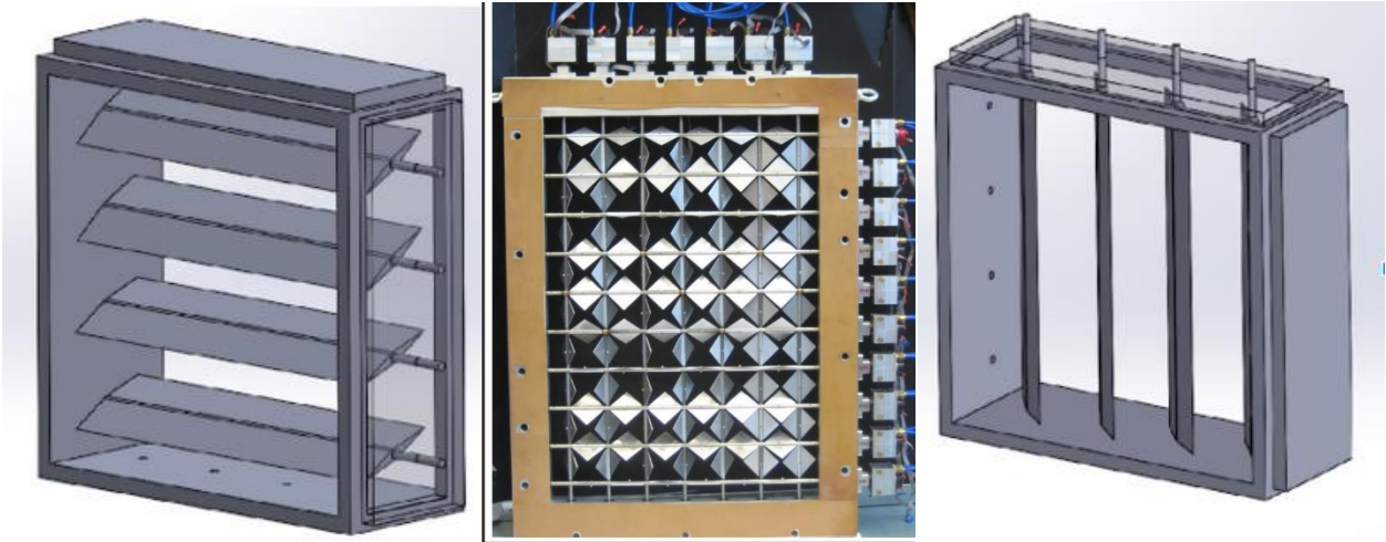
Figure 4: Left-horizontally aligned shutters; Center-rhomboid-grid shutters; Right- vertically aligned shutters
