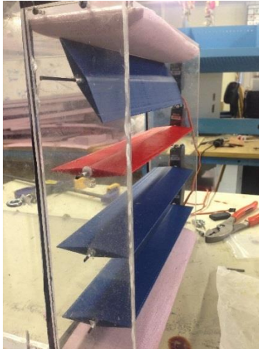
Figure 25: Shutter system acrylic frame
