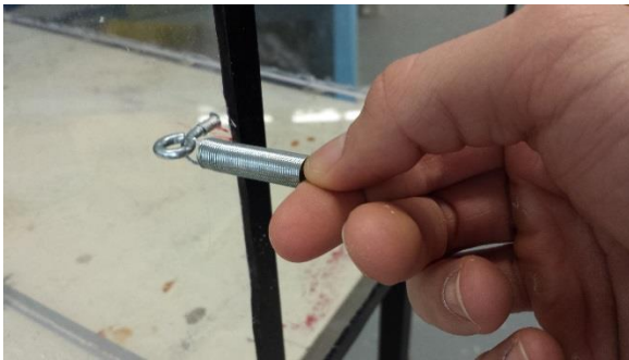
Figure 20: Spring attachment, not tensioned
