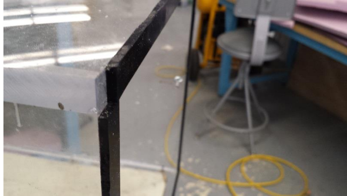
Figure 17: Rubber gasket used to line test section connecting edges
