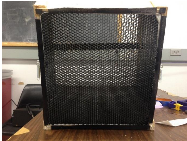
Figure 9: Second honeycomb structure, located at end of contraction section
