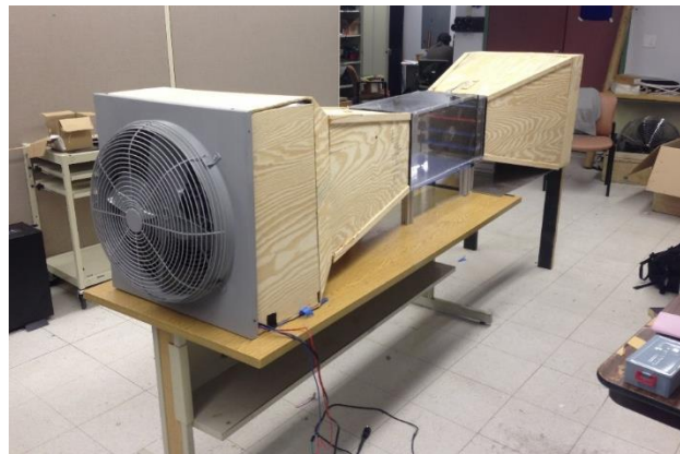
Figure 22: Fully assembled wind tunnel structure
