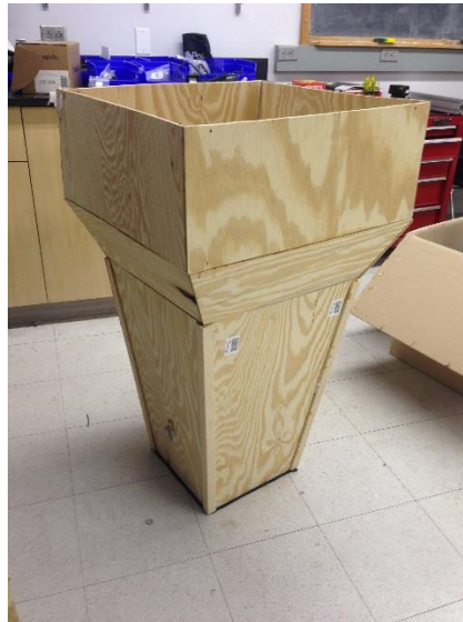
Figure 18: Completed wind tunnel diffusing section
