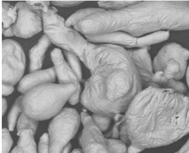
Figure V-19: SEM image at 1000X magnification to evaluate physical appearance of Zn prior to discharge.
