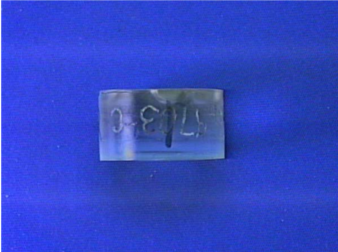
Figure IV-2: Side view of a cross-sectioned and polished Size 13 mount.
