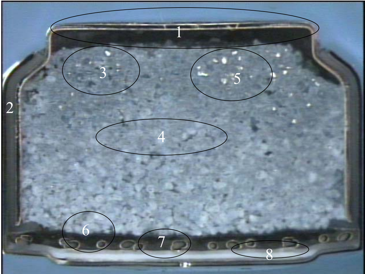
Figure V-10: Cross-sectional image of size 13 Zn/Air cell discharged at 1mA continuous current obtained via digital light microscopy.
