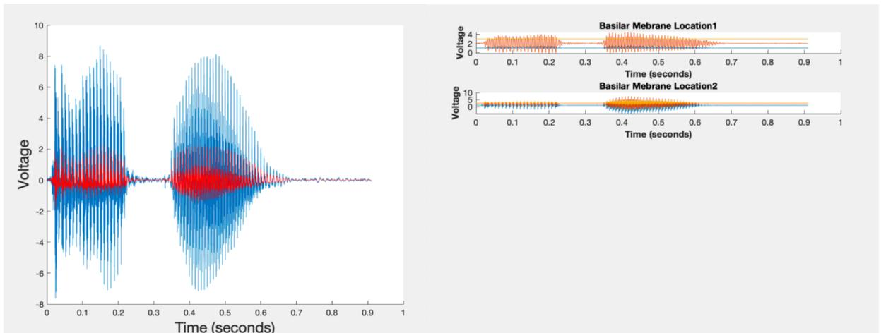
Figure 19: Inner Hair Cell Outputs. The graph on the left panel displays the input waveform in red, and the summed outputs of each inner hair cell in blue. The graph on the right panel displays the inner hair cell outputs that correspond to the first two basilar membrane locations for Simulation 2A. Both Location 1 and Location 2 have three inner hair cells receiving the same input signal from that location's output.
