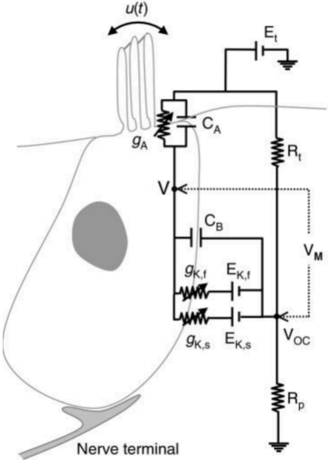
Figure 4: A circuit diagram of the Lopez-Poveda-Eustaquio-Martín model [12].
