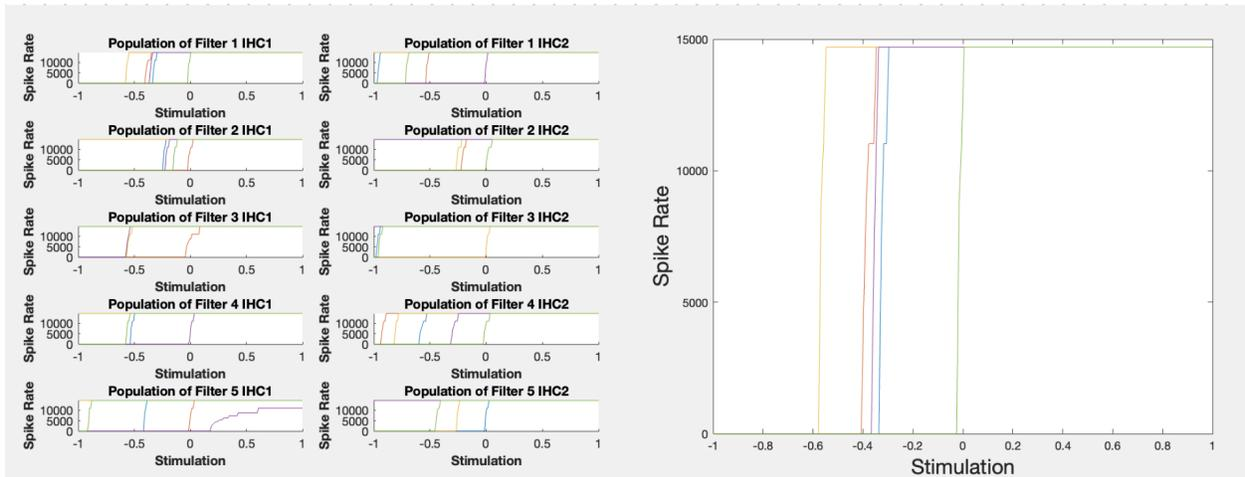
Figure 14: Activation Functions. The left panel displays the activation functions for the first 10 neural populations, with each function corresponding to one of the five neurons in each population. The right panel highlights the graph of the activations for one neural population.
