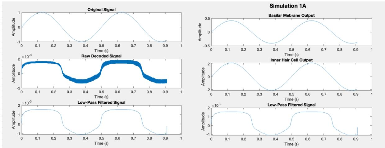
*Figure 15: Model Outputs. The graph displayed on the left panel compares the original input signal to the raw signal decoded by the auditory nerve to the final low pass filtered signal output to reduce high frequency noise. The graph displayed on the right panel compares the signal at the 3 major checkpoints throughout the model: Basilar Membrane Output, Inner Hair Cell Output, and Final Low Pass Filtered Decoded Signal.*
