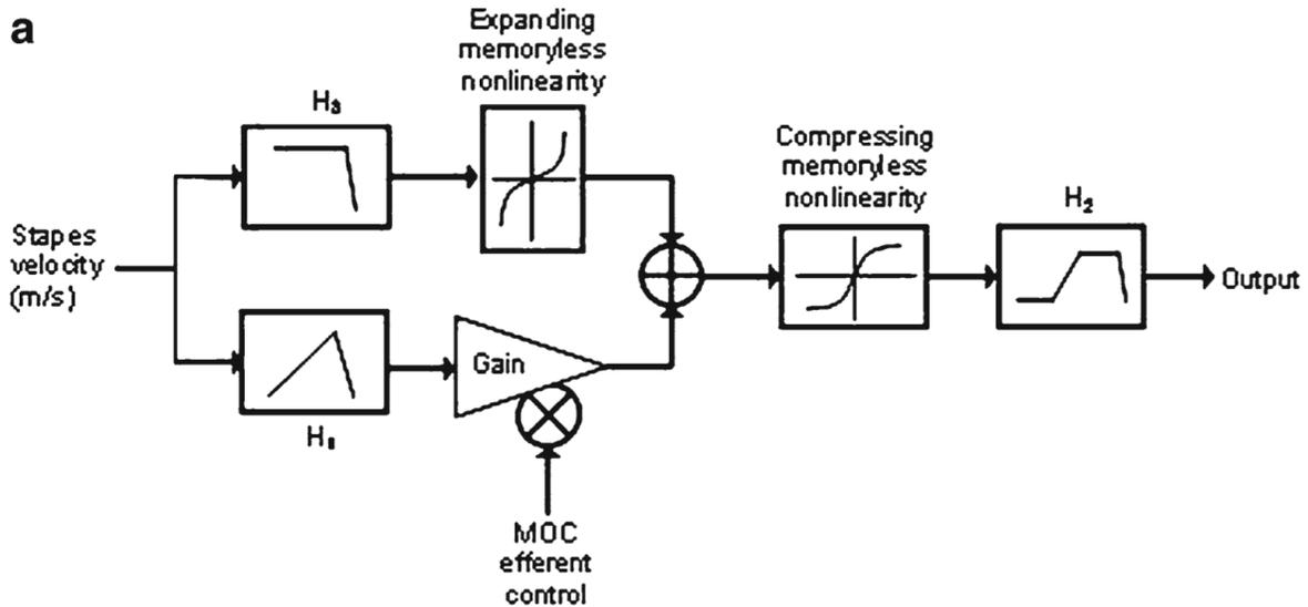
*Figure 3: Goldstein's Multiple BandPass NonLinear Model [11]*
