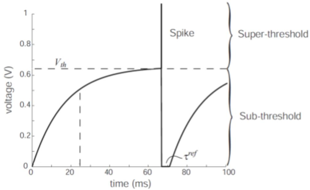
Figure 5: Spiking behavior of LIF neurons from the Neural Engineering Framework [6]
