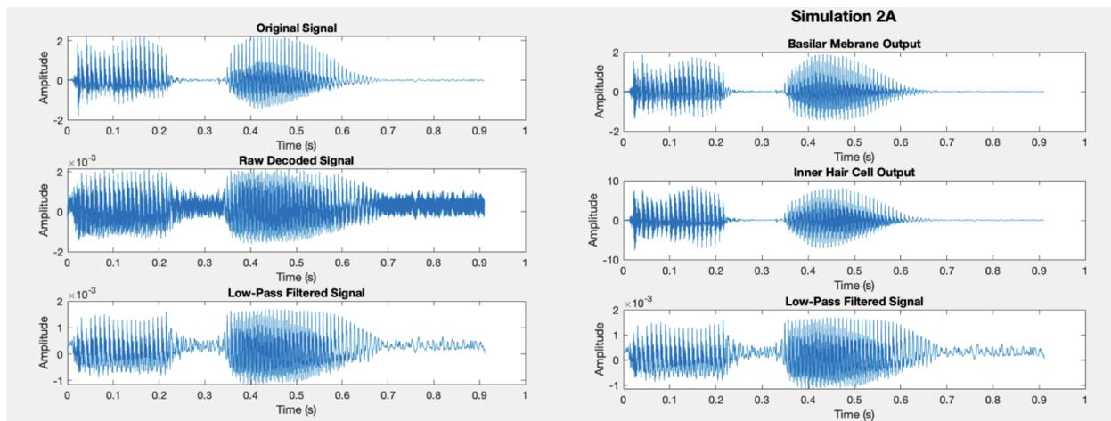
*Figure 21: Model Outputs. The graph displayed on the left panel compares the original input signal to the raw signal decoded by the auditory nerve to the final low pass filtered signal output to reduce high frequency noise. The graph displayed on the right panel compares the signal at the 3 major checkpoints throughout the model: Basilar Membrane Output, Inner Hair Cell Output, and Final Low Pass Filtered Decoded Signal.*
