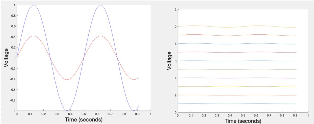
*Figure 10: Basilar Membrane Outputs. The graph on the left panel displays the input wave signal in blue, and the summed outputs of each basilar membrane channel in red. The graph on the right panel displays the output of each filter channel after filtering the input signal. The channels outputs at the bottom of the graph represent locations closer to the base of the basilar membrane (lower center frequency) and channels closer to the apex are higher on the graph (higher center frequency).*
