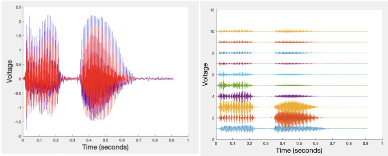
*Figure 18: Basilar Membrane Outputs. The graph on the left panel displays the input wave signal in blue, and the summed outputs of each basilar membrane channel in red. The graph on the right panel displays the output of each filter channel after filtering the input signal. The channels outputs at the bottom of the graph represent locations closer to the base of the basilar membrane (lower center frequency) and channels closer to the apex are higher on the graph (higher center frequency).*
