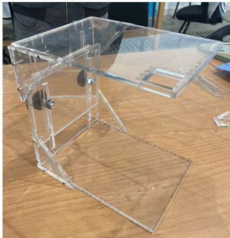
Figure 4. Completed SmartScan platform constructed of plexiglass
