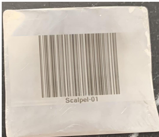
Figure 14. Square piece of stainless steel metal with a laser engraved barcode for demonstration purposes.
