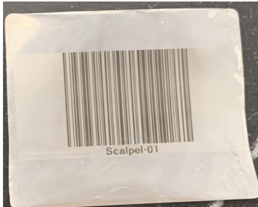
Figure 3. Square piece of stainless steel metal with a laser engraved barcode for demonstration purposes.
