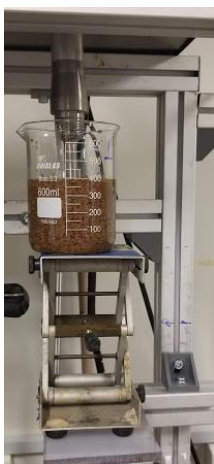
Figure 4: Set-up with ultrasonic probe for pretreatment of water and barley bagasse mixture.
