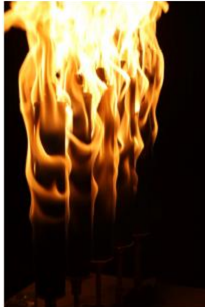
Figure 12 - Sample Flame of Cylindrical Port Burner
