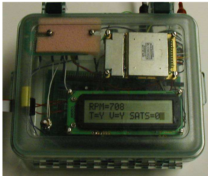
Figure 38: Device Displaying RPM in Real Time
