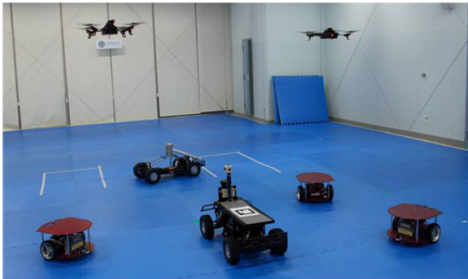
Figure 5.1: An example of a collaborative network consisting of ground and aerial vehicles. Data is relayed from/to the aerial vehicle to/from the ground vehicle to obtain more reliable information and greater accuracy about the vehicles' surroundings [4]. This network is very well suited to using agnostic video sources because it opens up for much more flexibility in its configuration - multiple combinations of these vehicles cooperating together can be achieved without defining new standards for each new vehicles video stream.
