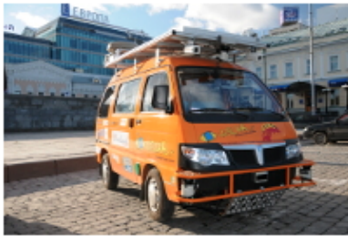
Vehicle for VIAC, Vislab Intercontinental Autonomous Challenge
