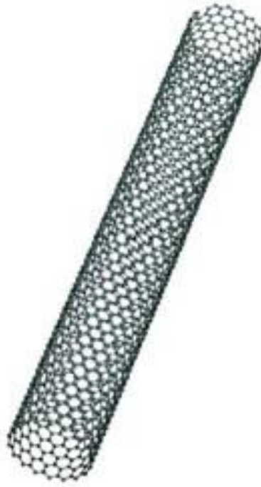
Figure 2-4: A Schematic of Single Wall Carbon Nanotube
