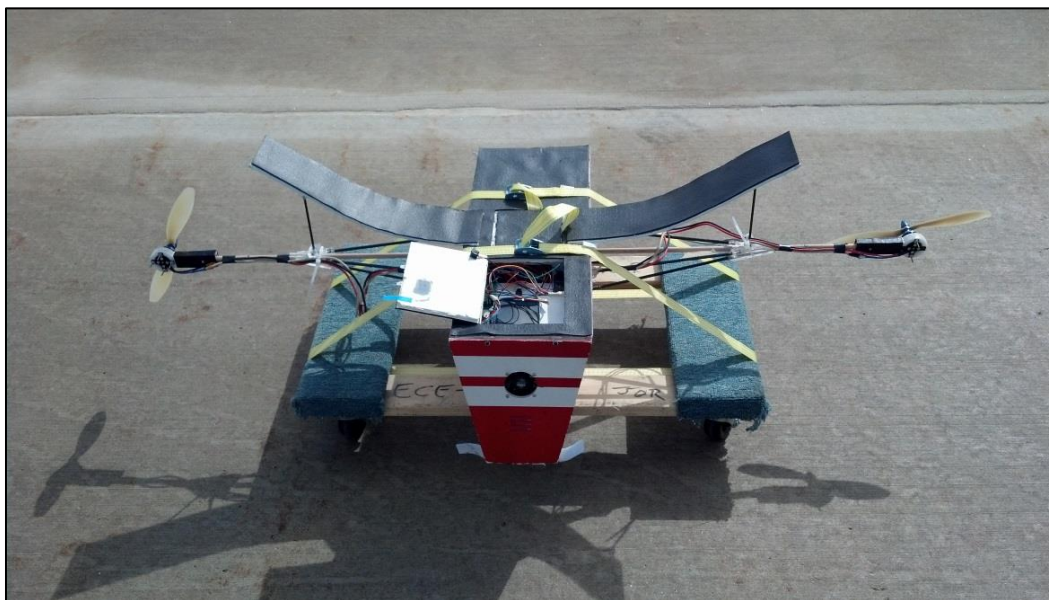
Figure 61: Gondola on Dolly for Ground Test
