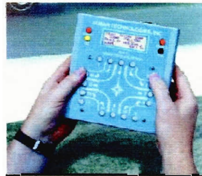
Figure 7: Electronic Turning Movement clicker made by JamarTech
