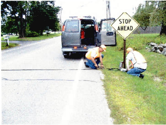
Figure 8: Traditional Automatic Traffic Recorders Being Placed
