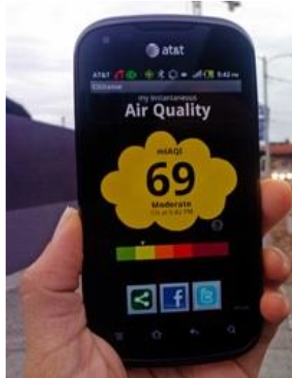
Figure.4 Smartphone displaying air quality readout
