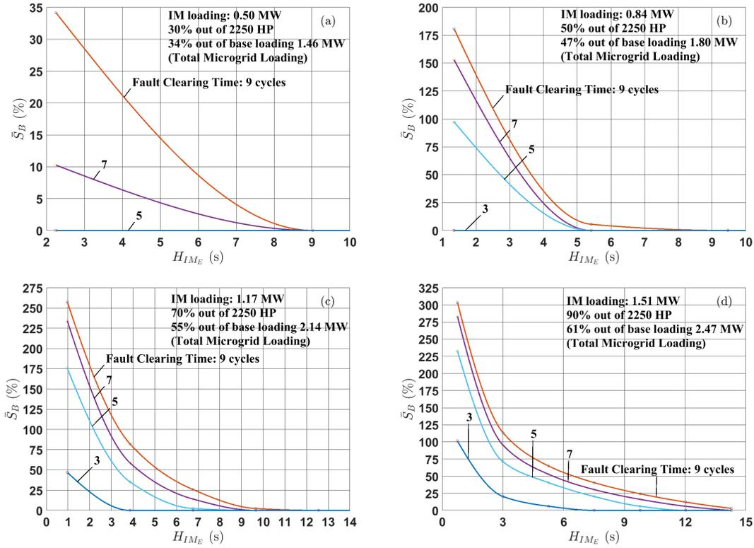
Figure 5.20: Normalized minimum BESS inverter size  $\bar{S}_B$  as a function of equivalent motor inertia constant  $H_{IME}$  with fault clearing time as the parameter: (a). 34 % IM loading, (b). 47 % IM loading, (c). 55 % IM loading, (d). 61 % IM loading.
