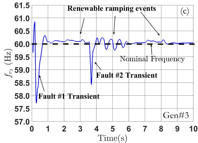
Figure 6.23: The synchronous generators rotor frequency  $f_r$  (Hz) vs. time under multiple faults and renewable generation ramping events with adaptive voltage regulation (no regulation delay): (a)  $f_{r_1}$ : 5 MVA hydroelectric generator; (b)  $f_{r_2}$ : 1.8 MVA diesel generator; (c)  $f_{r_3}$ : 3.125 MVA diesel generator
