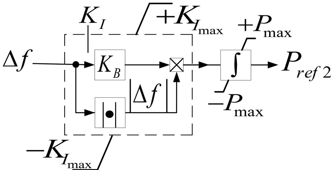
Figure 4.4: Adaptive Secondary Frequency Controller Block Diagram
