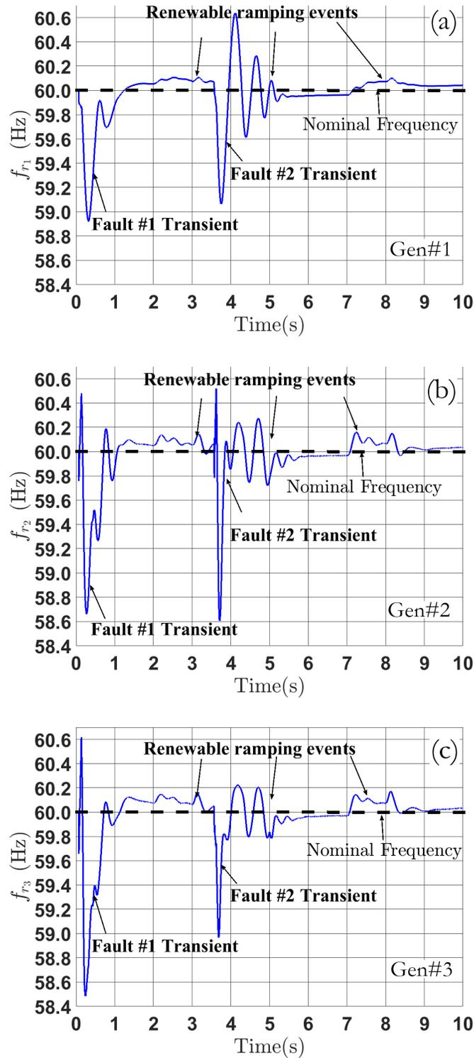
Figure 6.19: The synchronous generators rotor frequency  $f_r$  (Hz) vs. time under multiple faults and renewable generation ramping events with normal voltage regulation: (a)  $f_{r_1}$ : 5 MVA hydroelectric generator; (b)  $f_{r_2}$ : 1.8 MVA diesel generator; (c)  $f_{r_3}$ : 3.125 MVA diesel generator
