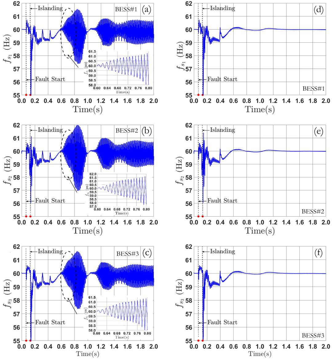
Figure 6.2: Estimated PLL Frequency  $f_s$ ; (left column): unstable under secondary controller with  $K_I = 3000$ , (right column): stable under secondary controller with adaptive gain using  $K_B = 3 \times 10^5$ : (a)  $f_{s1}$ , unstable; (b)  $f_{s2}$ , unstable; (c)  $f_{s3}$ , unstable; (d)  $f_{s1}$ , stable; (e)  $f_{s2}$ , stable; (f)  $f_{s3}$ , stable
