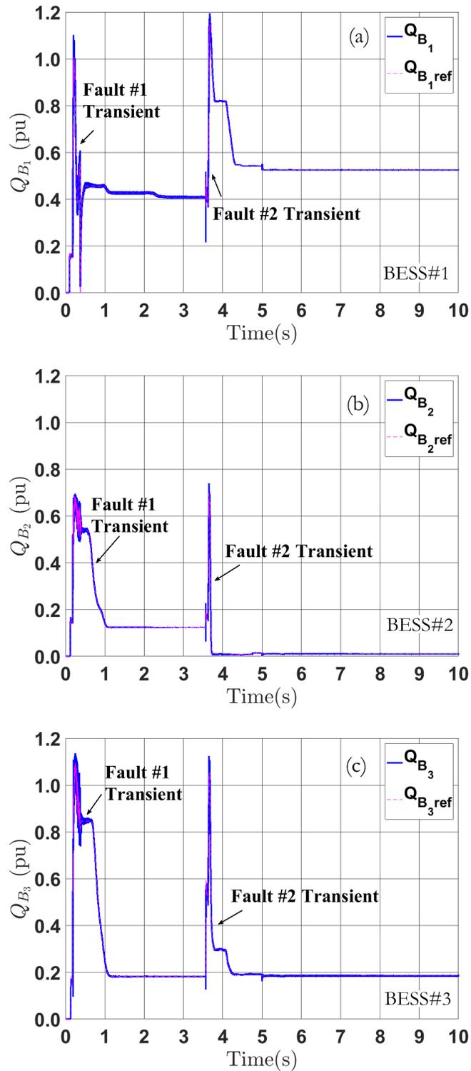
Figure 6.30: BESSs reactive power vs. time under multiple faults and renewable generation ramping events with adaptive voltage regulation (no regulation delay): (a)  $Q_{B_1}$ ; (b)  $Q_{B_2}$ ; (c)  $Q_{B_3}$
