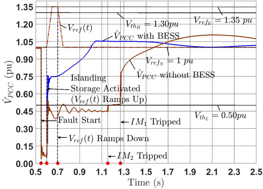
Figure 5.23:  $\hat{V}_{PCC}$  with and without 3.1 MVA BESS
