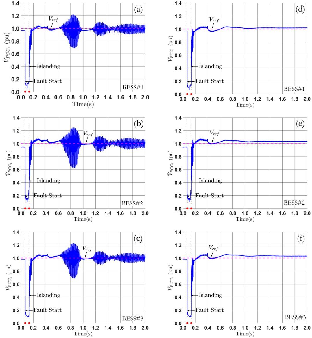
Figure 6.4: The PCCs voltage magnitude  $\hat{V}_{PCC}$  vs. time; (left column): unstable under secondary controller with  $K_I = 3000$ , (right column): stable under secondary controller with adaptive gain using  $K_B = 3 \times 10^5$ : (a)  $\hat{V}_{PCC_1}$ , unstable; (b)  $\hat{V}_{PCC_2}$ , unstable; (c)  $\hat{V}_{PCC_3}$ , unstable; (d)  $\hat{V}_{PCC_1}$ , stable; (e)  $\hat{V}_{PCC_2}$ , stable; (f)  $\hat{V}_{PCC_3}$ , stable
