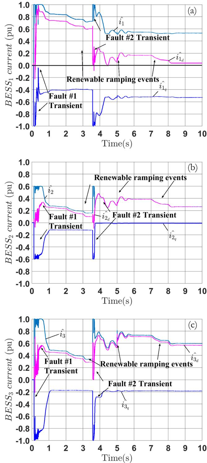
Figure 6.28: BESSs current magnitudes transients under multiple faults and renewable generation ramping events with adaptive voltage regulation (no regulation delay): (a) BESS<sub>1</sub>; (b) BESS<sub>2</sub>; (c) BESS<sub>3</sub>
