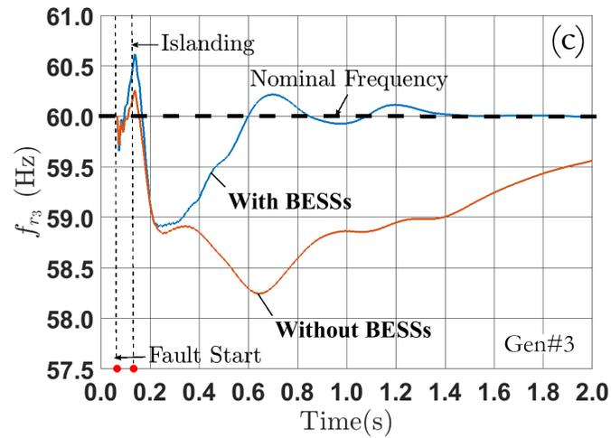
Figure 6.6: The synchronous generators rotor frequency  $f_r$  (Hz) vs. time; with and without BESSs: (a)  $f_{r_1}$ : 5 MVA hydroelectric generator; (b)  $f_{r_2}$ : 1.8 MVA diesel generator; (c)  $f_{r_3}$ : 3.125 MVA diesel generator
