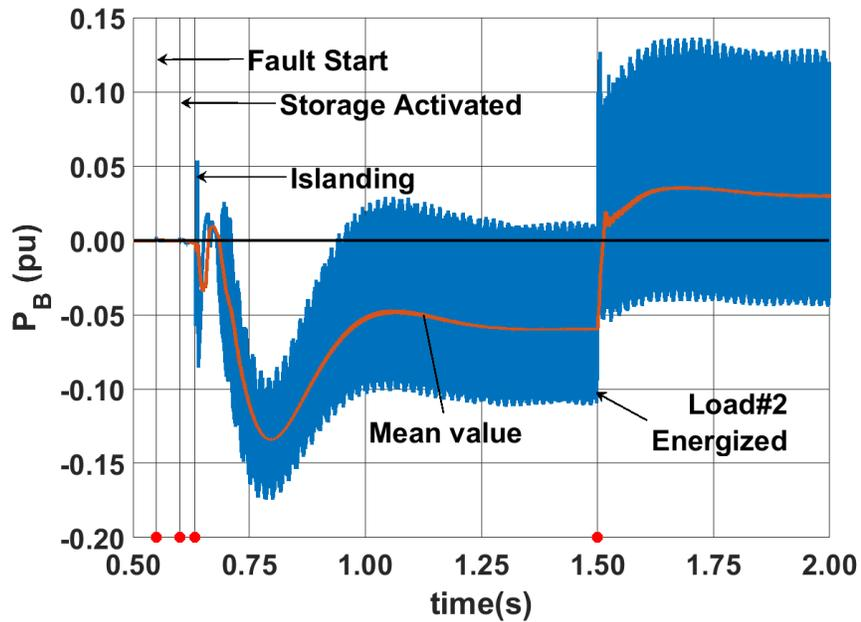
Figure 4.7: Unstable control performance: The BESS power vs. time for linear droop with  $R_c = 1\%$  and secondary controller gain of 1000.
