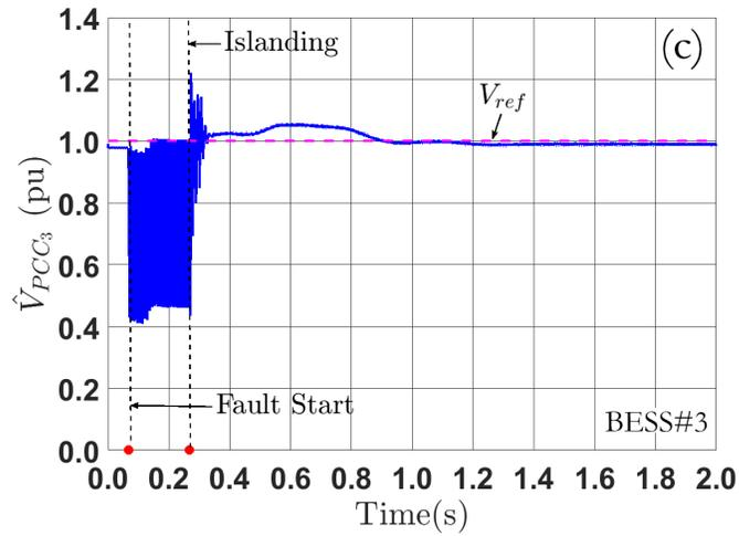
Figure 6.12: The PCCs voltage magnitude  $\hat{V}_{PCC}$  vs. time under 12 cycles *asymmetrical* fault: (a)  $\hat{V}_{PCC_1}$ ; (b)  $\hat{V}_{PCC_2}$ ; (c)  $\hat{V}_{PCC_3}$
