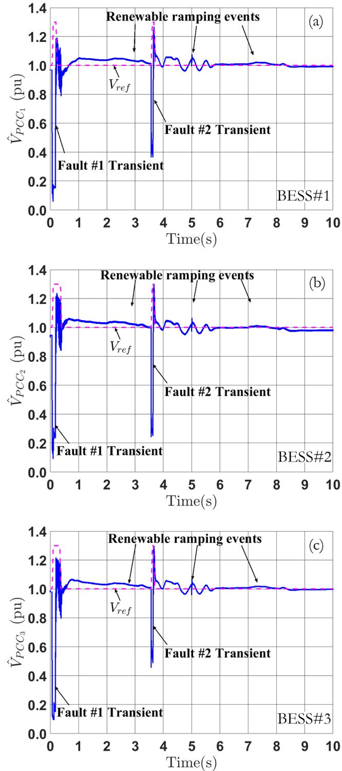
Figure 6.24: The PCCs voltage magnitude  $\hat{V}_{PCC}$  vs. time under multiple faults and renewable generation ramping events with adaptive voltage regulation (no regulation delay): (a)  $\hat{V}_{PCC_1}$ ; (b)  $\hat{V}_{PCC_2}$ ; (c)  $\hat{V}_{PCC_3}$
