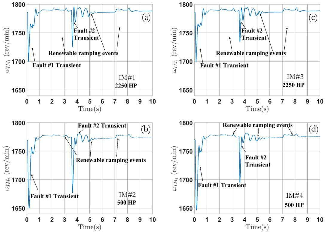
Figure 6.18: Induction motors speed  $\omega_{IM}$  vs. time, under multiple faults and renewable generation ramping events with normal voltage regulation: (a)  $\omega_{IM_1}$ : 2250 HP; (b)  $\omega_{IM_2}$ : 500 HP; (c)  $\omega_{IM_3}$ : 2250 HP; (d)  $\omega_{IM_4}$ : 500 HP
