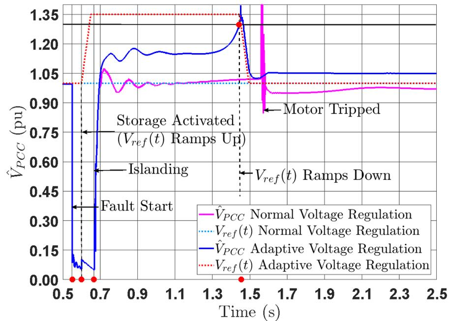
Figure 5.16:  $\hat{V}_{PCC}$  with and without adaptive voltage regulation
