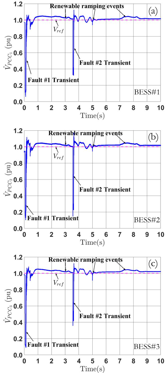
Figure 6.20: The PCCs voltage magnitude  $\hat{V}_{PCC}$  vs. time under multiple faults and renewable generation ramping events with normal voltage regulation: (a)  $\hat{V}_{PCC_1}$ ; (b)  $\hat{V}_{PCC_2}$ ; (c)  $\hat{V}_{PCC_3}$
