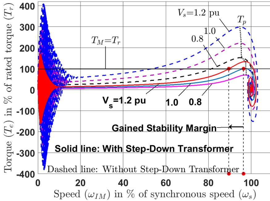
Figure 5.3: Induction motor free accelerating torque-speed curves
