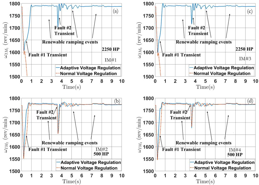
Figure 6.26: Induction motors speed  $\omega_{IM}$  vs. time, under multiple faults and renewable generation ramping events with adaptive voltage regulation (no regulation delay): (a)  $\omega_{IM_1}$ : 2250 HP; (b)  $\omega_{IM_2}$ : 500 HP; (c)  $\omega_{IM_3}$ : 2250 HP; (d)  $\omega_{IM_4}$ : 500 HP
