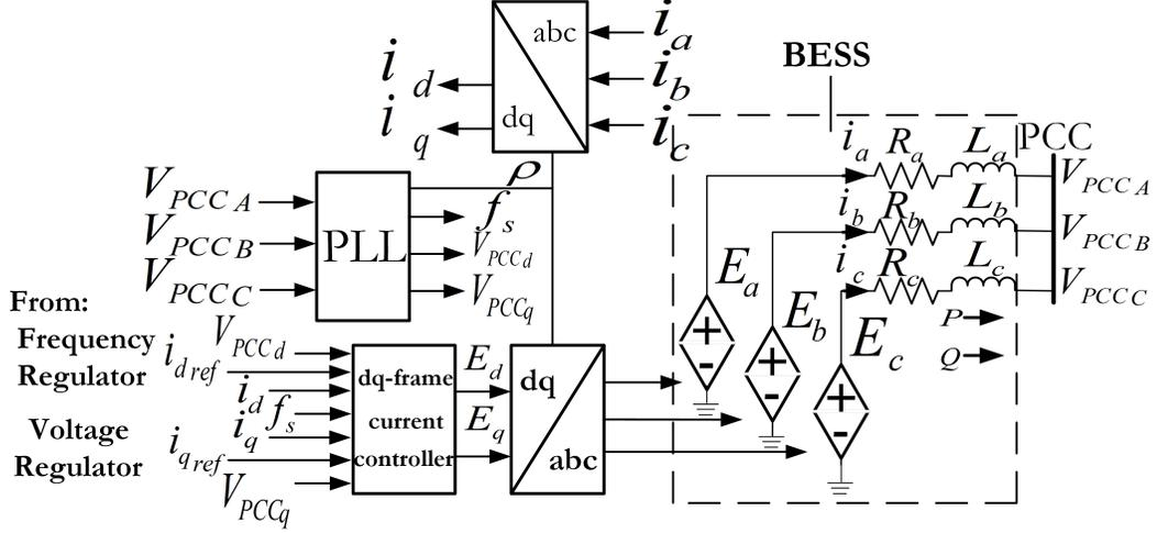
Figure 3.7: Overall converter modeling and control block diagrams
