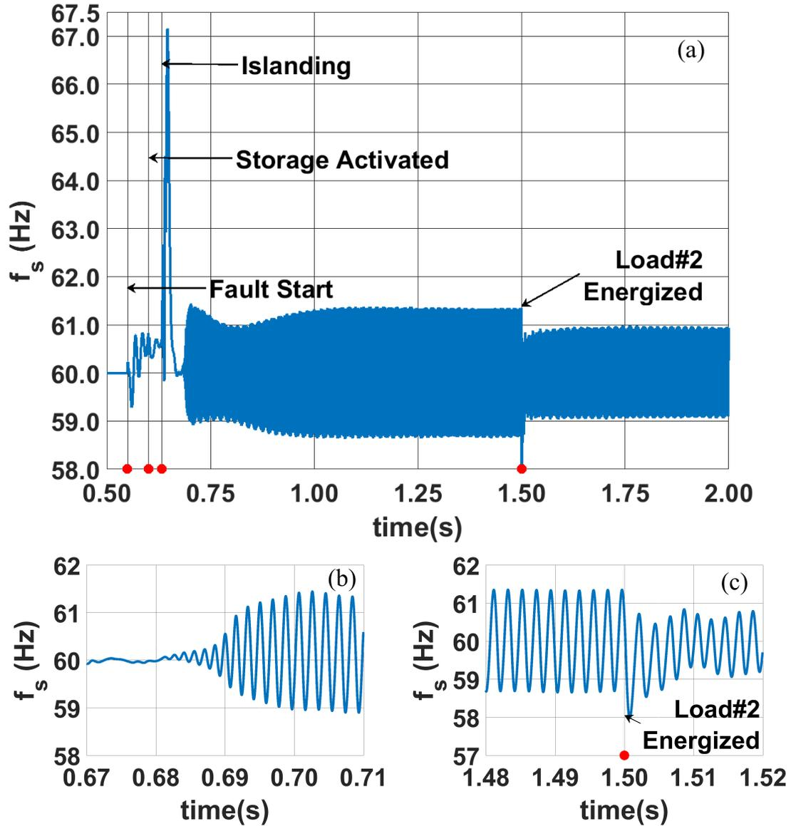
Figure 4.5: Estimated PLL frequency  $f_s$  for linear droop with  $R_c = 1\%$  and secondary controller gain of 1000: (a). Overall unstable response, (b). Magnified oscillogram for  $0.67 < t < 0.71$  s, (c). Magnified oscillogram for  $1.48 < t < 1.52$  s.
