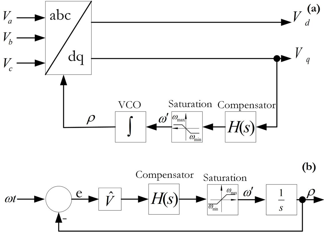
Figure A.4: PLL schematic and associated control block diagram
