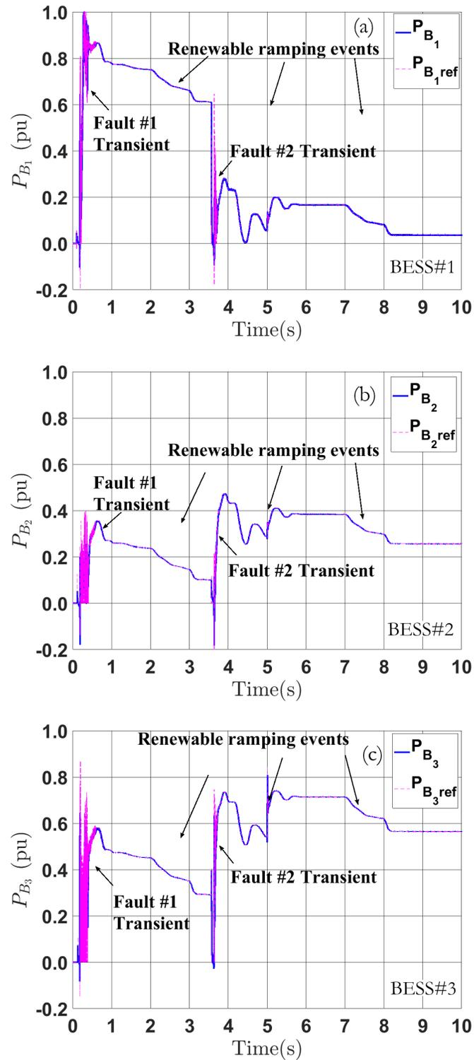
Figure 6.29: BESSs real power vs. time under multiple faults and renewable generation ramping events with adaptive voltage regulation (no regulation delay): (a)  $P_{B_1}$ ; (b)  $P_{B_2}$ ; (c)  $P_{B_3}$
