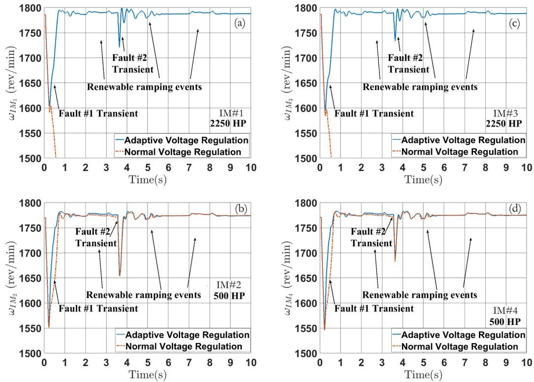
Figure 6.32: Induction motors speed  $\omega_{IM}$  vs. time, under multiple faults and renewable generation ramping events with adaptive voltage regulation (including regulation delay): (a)  $\omega_{IM_1}$ : 2250 HP; (b)  $\omega_{IM_2}$ : 500 HP; (c)  $\omega_{IM_3}$ : 2250 HP; (d)  $\omega_{IM_4}$ : 500 HP
