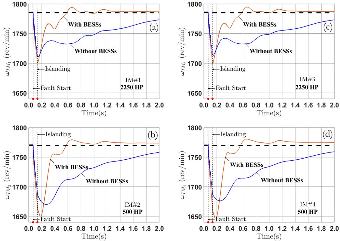
Figure 6.7: Induction motors speed  $\omega_{IM}$  vs. time, with and without BESSs: (a)  $\omega_{IM_1}$ : 2250 HP; (b)  $\omega_{IM_2}$ : 500 HP; (c)  $\omega_{IM_3}$ : 2250 HP; (d)  $\omega_{IM_4}$ : 500 HP
