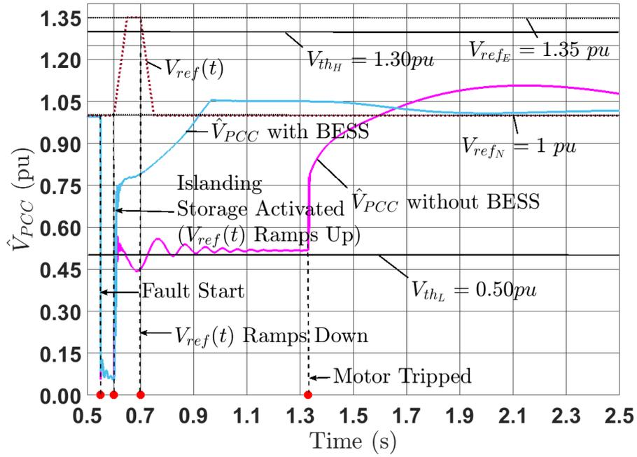
Figure 5.9:  $\hat{V}_{PCC}$  with and without 2.5 MVA BESS
