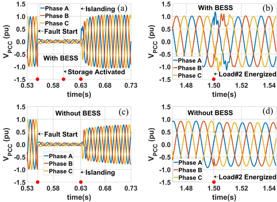
Figure 4.11: Magnified PCC voltage oscillogram vs. time: (a). With BESS adaptive control, for  $0.53 < t < 0.73s$ , (b). With BESS adaptive control, for load#2 switched in at  $t = 1.5s$ , (c). Without BESS, for  $0.53 < t < 0.73s$ , (d). Without BESS, for load#2 switched in at  $t = 1.5s$ .
