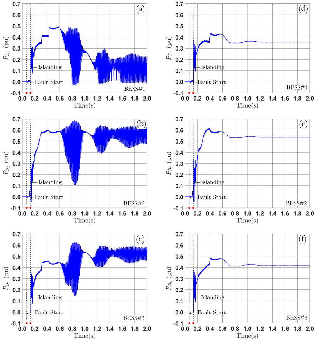
Figure 6.3: The BESSs power vs. time; (left column): unstable under secondary controller with  $K_I = 3000$ , (right column): stable under secondary controller with adaptive gain using  $K_B = 3 \times 10^5$ : (a)  $P_{B_1}$ , unstable; (b)  $P_{B_2}$ , unstable; (c)  $P_{B_3}$ , unstable; (d)  $P_{B_1}$ , stable; (e)  $P_{B_2}$ , stable; (f)  $P_{B_3}$ , stable
