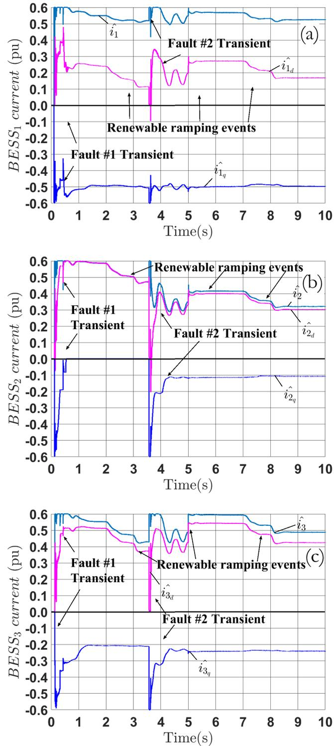
Figure 6.15: BESSs current magnitudes transients under multiple faults and renewable generation ramping events with normal voltage regulation: (a) BESS<sub>1</sub>; (b) BESS<sub>2</sub>; (c) BESS<sub>3</sub>
