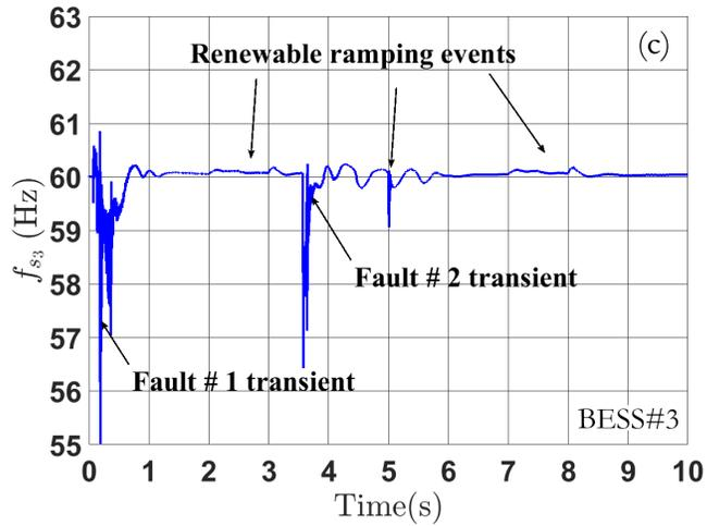
Figure 6.27: Estimated PLL Frequency  $f_s$  under multiple faults and renewable generation ramping events with adaptive voltage regulation (no regulation delay): (a)  $f_{s_1}$ ; (b)  $f_{s_2}$ ; (c)  $f_{s_3}$
