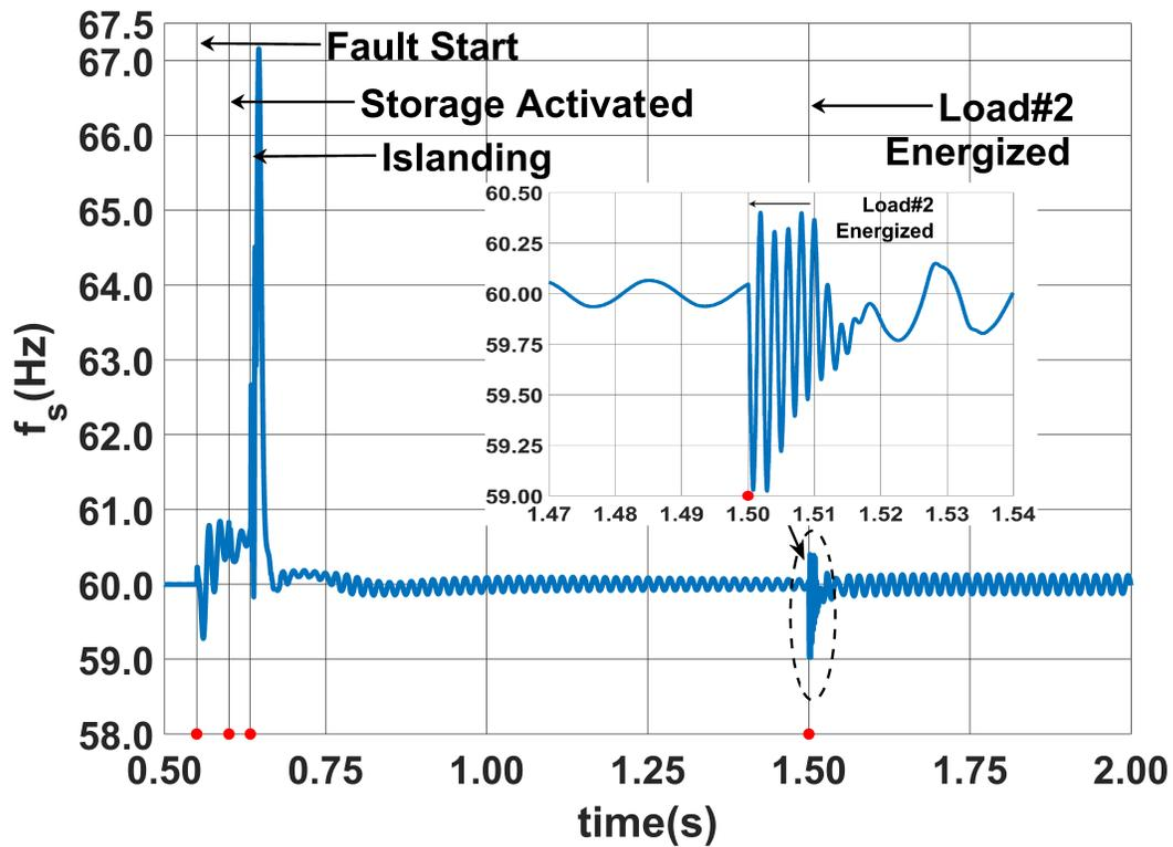
Figure 4.8: Estimated PLL frequency  $f_s$  for adaptive nonlinear droop with  $R_c = 1\%$  and secondary controller gain of 1000.
