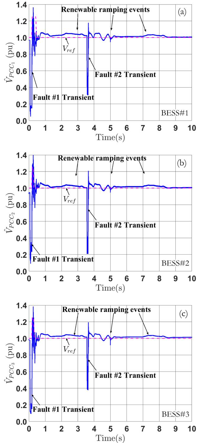
Figure 6.31: The PCCs voltage magnitude  $\hat{V}_{PCC}$  vs. time under multiple faults and renewable generation ramping events with adaptive voltage regulation (including regulation delay): (a)  $\hat{V}_{PCC_1}$ ; (b)  $\hat{V}_{PCC_2}$ ; (c)  $\hat{V}_{PCC_3}$
