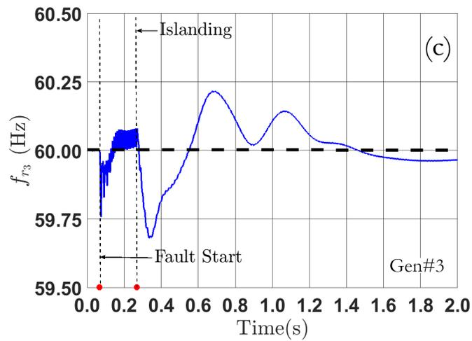
Figure 6.11: The synchronous generators rotor frequency  $f_r$  (Hz) vs. time under 12 cycles *asymmetrical* fault: (a)  $f_{r_1}$ : 5 MVA hydroelectric generator; (b)  $f_{r_2}$ : 1.8 MVA diesel generator; (c)  $f_{r_3}$ : 3.125 MVA diesel generator
