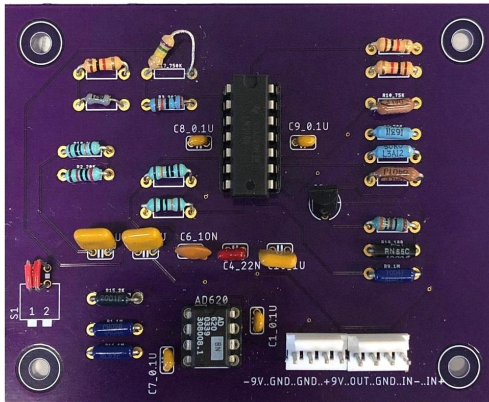
Figure 5.85: The finished PCB for the ECG Wireless Circuit
