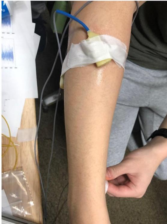
*Figure 5.39: Electrode Placement for Testing Wired EMG using Prosthetic Hand*
