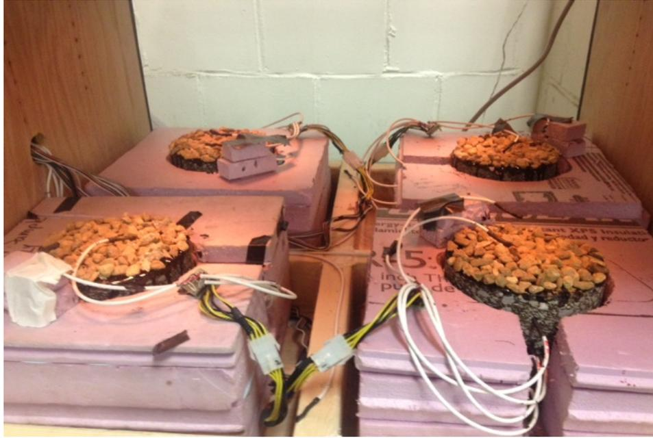
**Figure 6: GRCS Surfaced Samples being tested (photo with sides removed) in the solar simulator**
