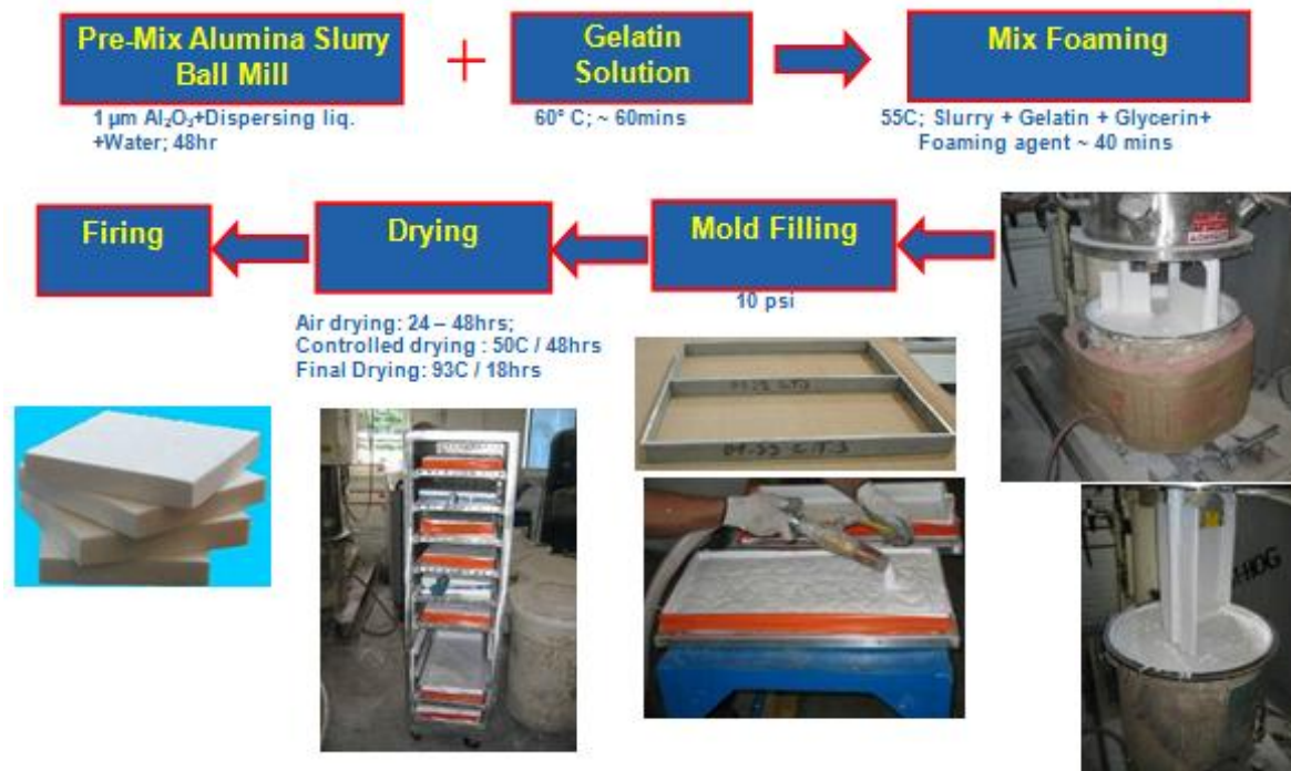
Figure 6: Alumina Foam Fabrication Process. [1]
