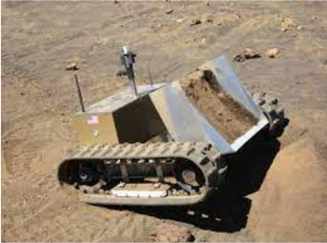
Figure 17: NASA Cratos undergoing testing on volcanic soil in Hawaii.
