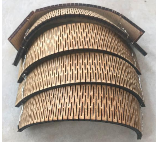
Figure 26: Completed Shoulder Pad Manufactured with Wood
