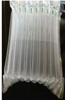
Figure 15: Ten-Inch-Long Bubble Wrap Tubes
