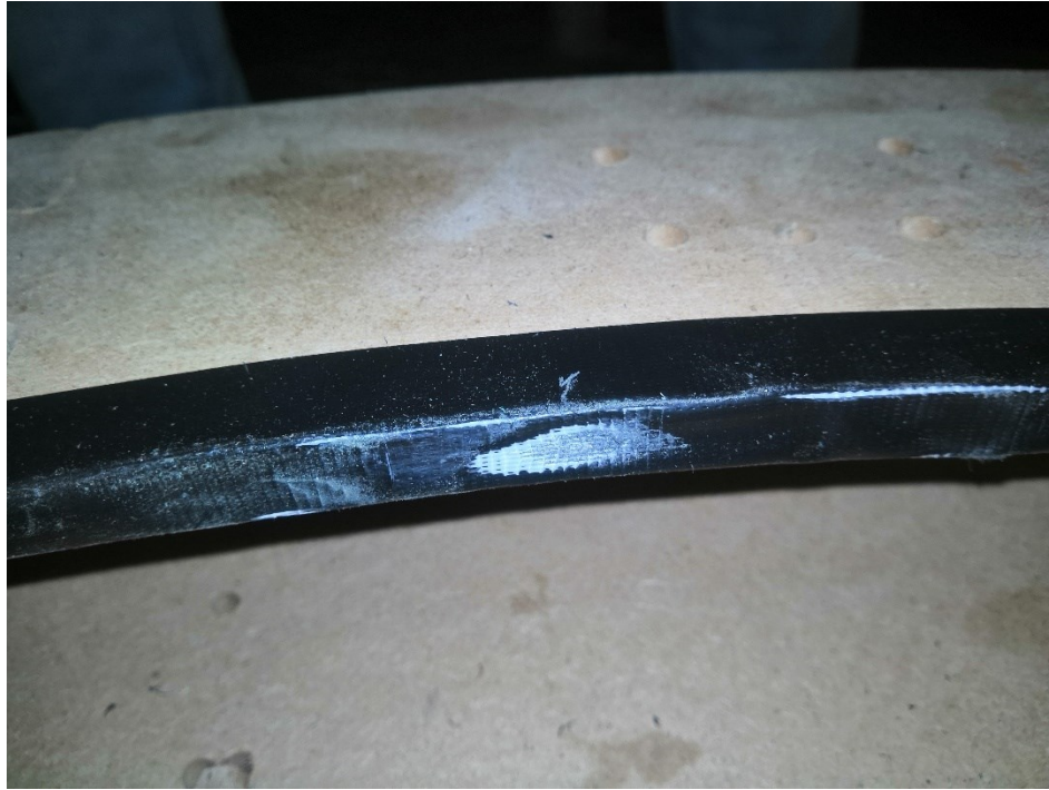
Figure 92: Rotating Ring Friction Material Wearing
