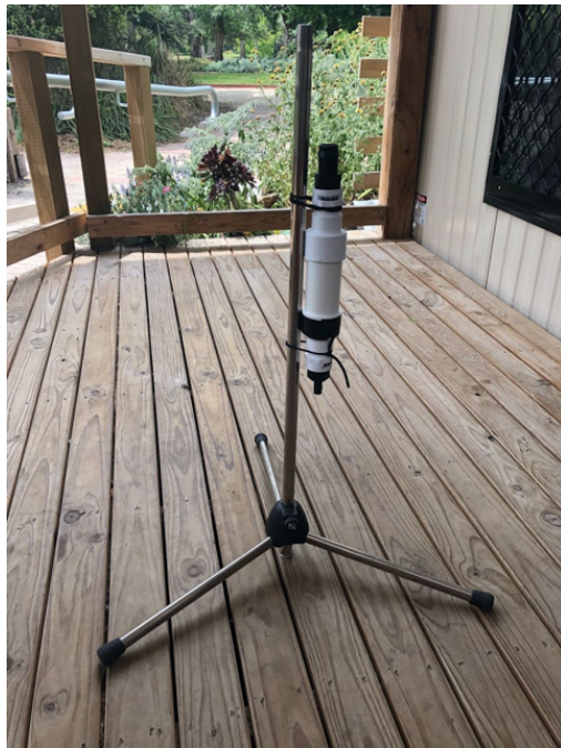
Figure 25. Tripod Fixture to Hold the Filter Upright.
