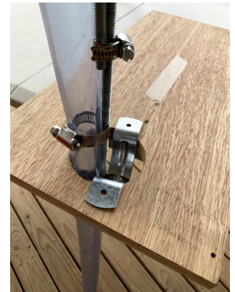
Figure 24. Stabilizing Base for the Inlet.
