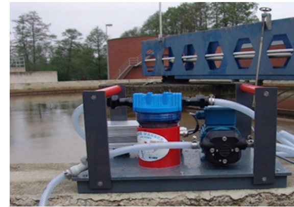
Figure 10. Above-Water Pump System (Mintenig, Int-Veen, Löder, Primpke, & Gerdts, 2017).
