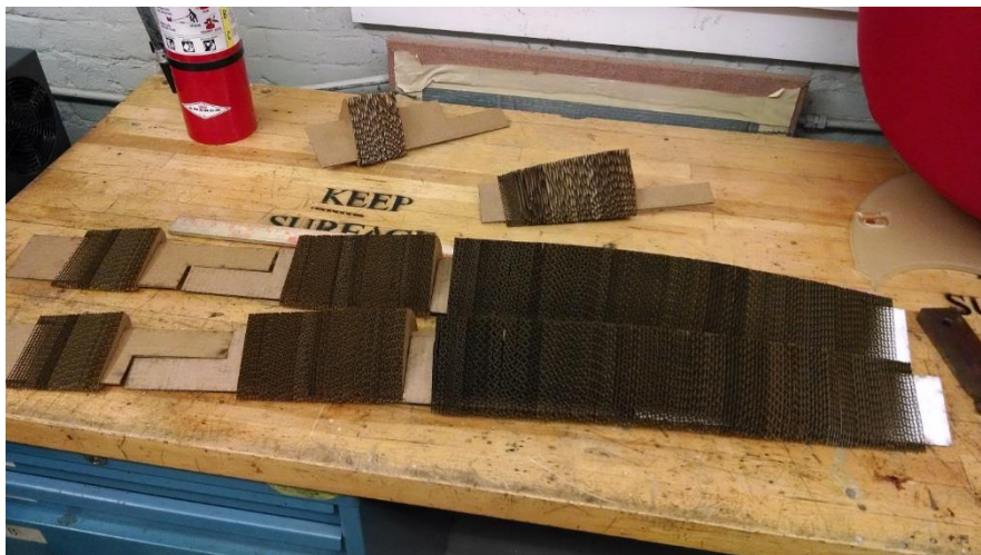
Figure 31 - The outrigger cross sections mid-assembly
