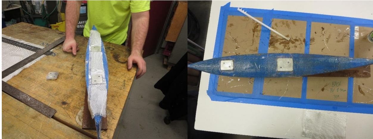
A. Fitting and planning fiberglass housing
