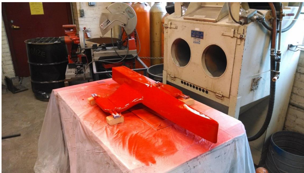
Figure 40 - Center hull with a fresh coat of paint
