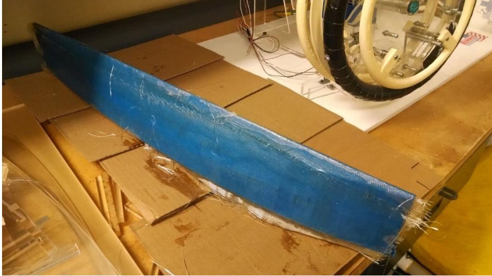
Figure 33 - First layer of fiberglass on the first outrigger.
