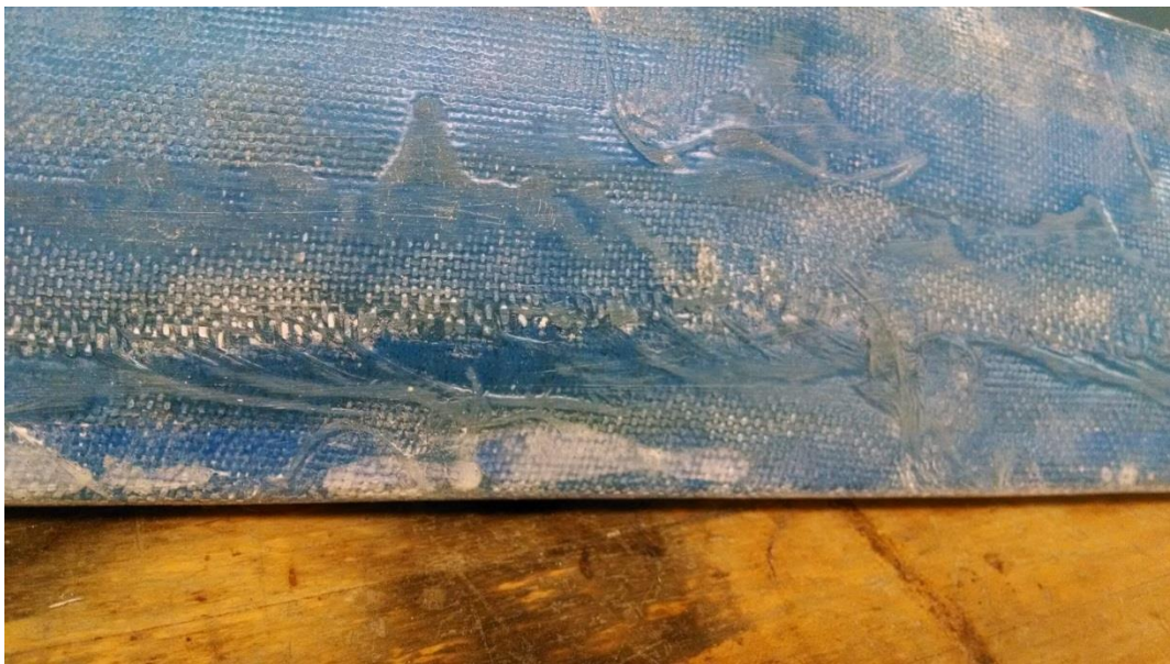
Figure 34 - Close up of sanded fiberglass threads.
