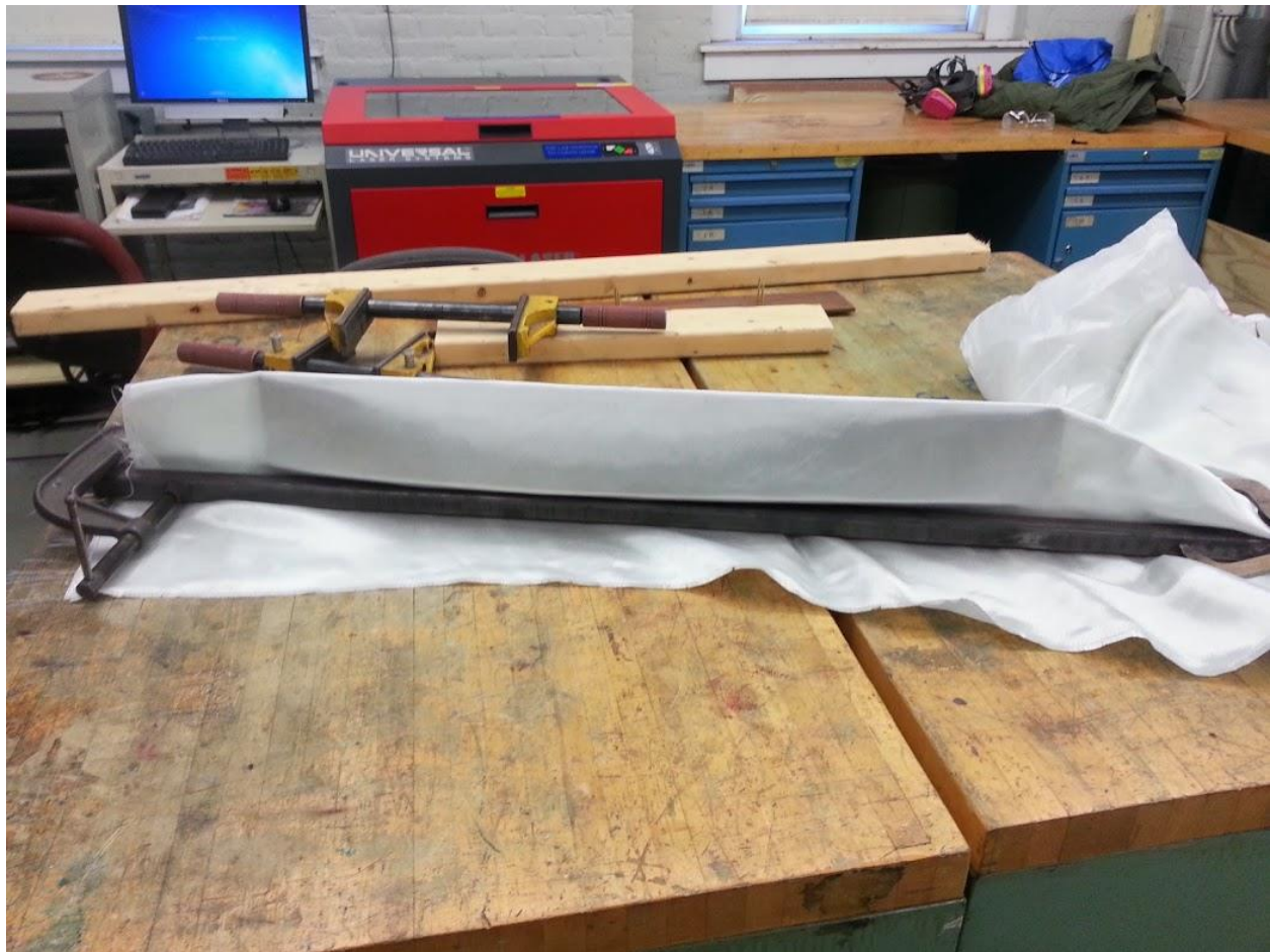
Figure 35 - Fiberglass stretched over hull and clamped in place.
