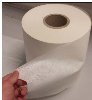
Figure A-13: Catalyst-embedded paper.
