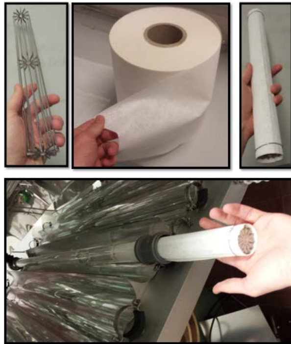
Figure 3.7: (From left to right) round steel holders, commercial grade \text{TiO}_2 catalyst embedded in porous paper, wrapped steel holders, holders being inserted into the chamber of the CPC reactor.
