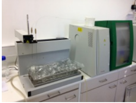
Figure A-14: TOC analyzer.
