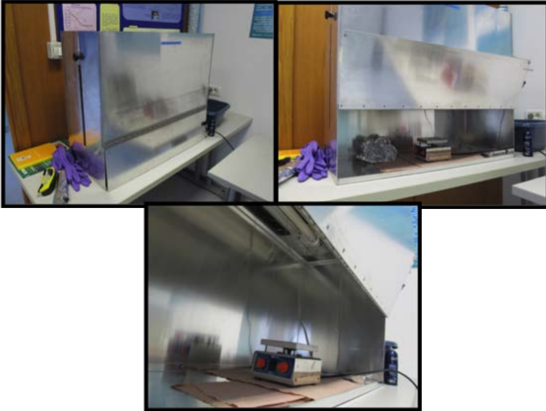
Figure 3.1: UV darkness box closed (top left), UV darkness box opened (top right), inside of UV darkness box with UV light source above stir plate (bottom).
