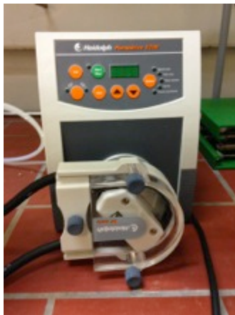
Figure A-9: Batch reactor pump.
