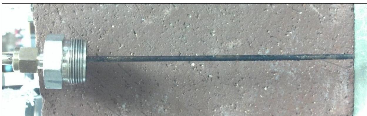
Figure 17: Helium gas inlet line
