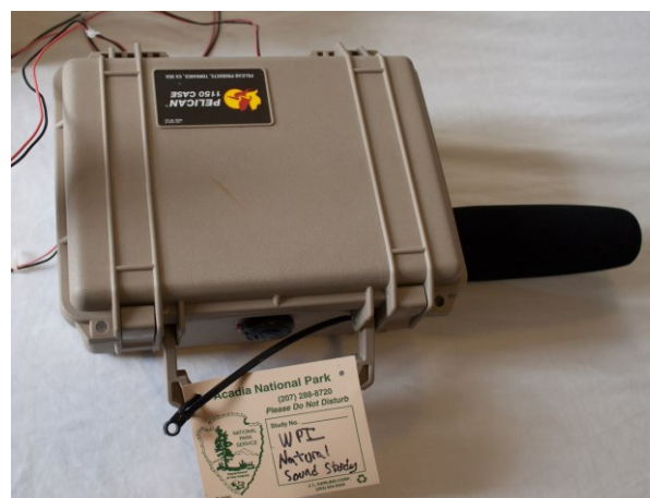
Figure 28: Waterproof Case Latched Closed
