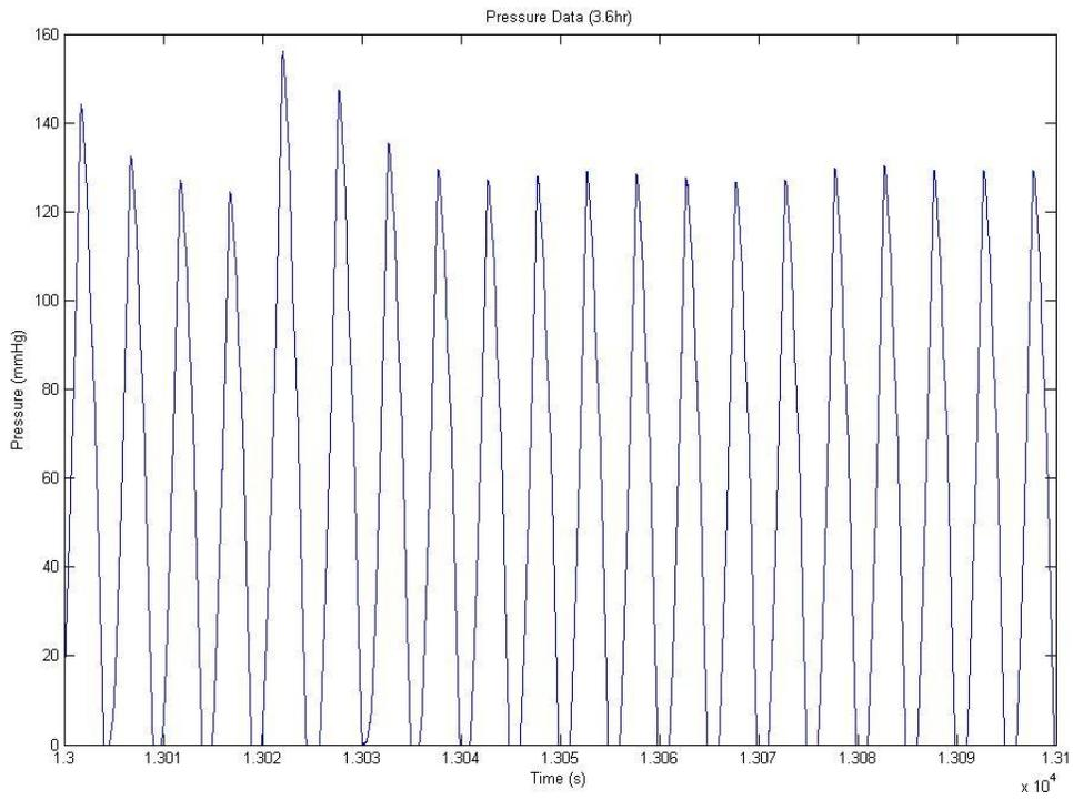
**Figure 21: Fatigue Test Pressure Data (3.6 hr)**
