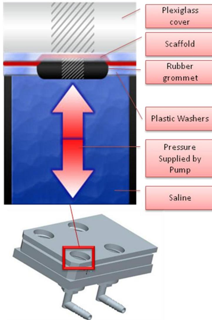
**Figure 7: Schematic of Fatigue Strength Experiment**
