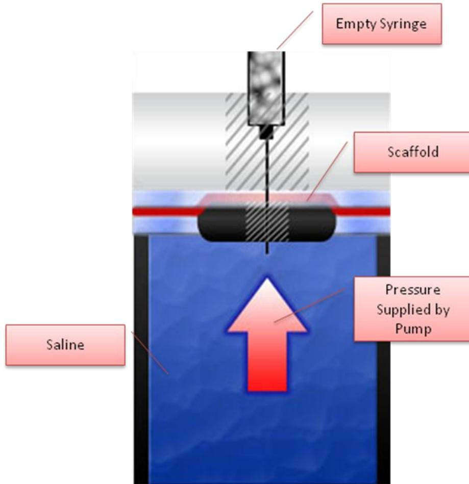
**Figure 6: Schematic of Self-Seal Experiment**
