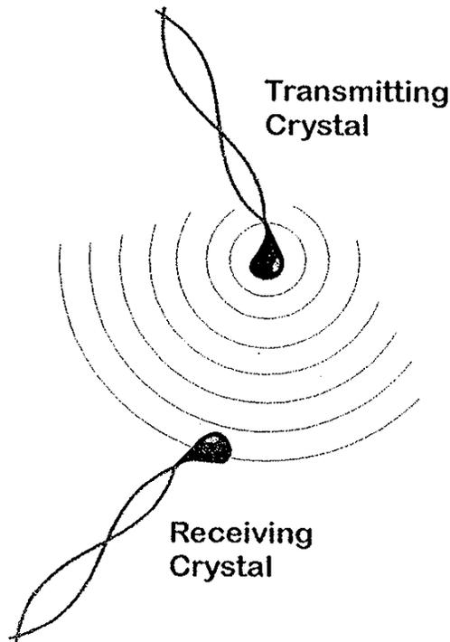
Figure 1 Ultrasonic Transmission and Reception Using Piezoelectric Transducers.
