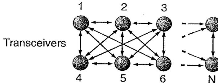
Figure 3 The Digital Sonomicrometer can measure distances between an array of crystals, when connected to transceivers.
