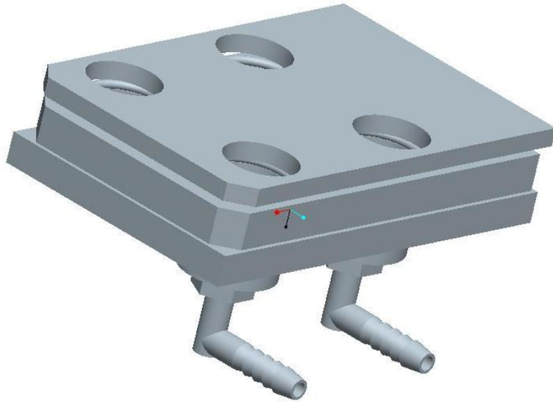
**Figure 5: Schematic of Fatigue Apparatus**
