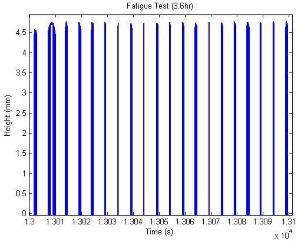
**Figure 20: Fatigue Test Displacement Data (3.6 hr)**
