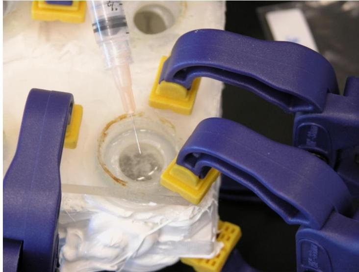
**Figure 10: UBM Self-Seal Test**
