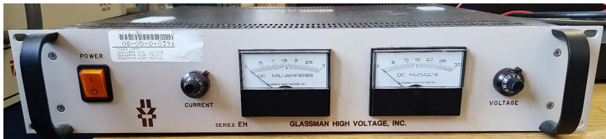
Figure 14: EHD High Voltage Supply Box
