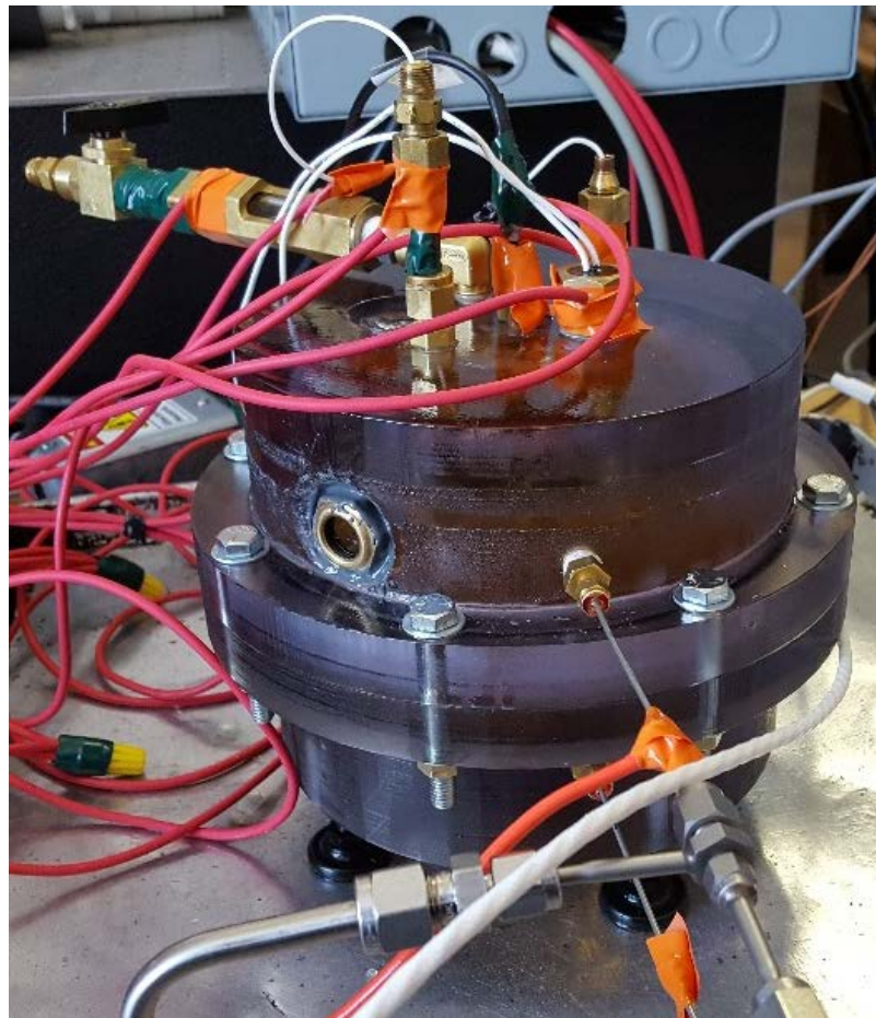
Figure 9: Assembled EHD Storage Tank ready for Experimentation
