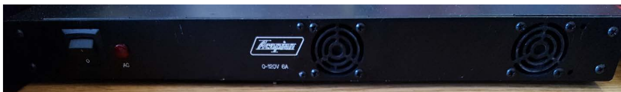
Figure 15: Heater Voltage Supply Box
