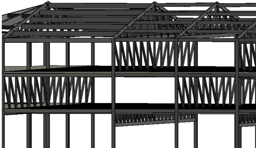
Figure 12: Staggered Truss System, Image from Autodesk Revit
