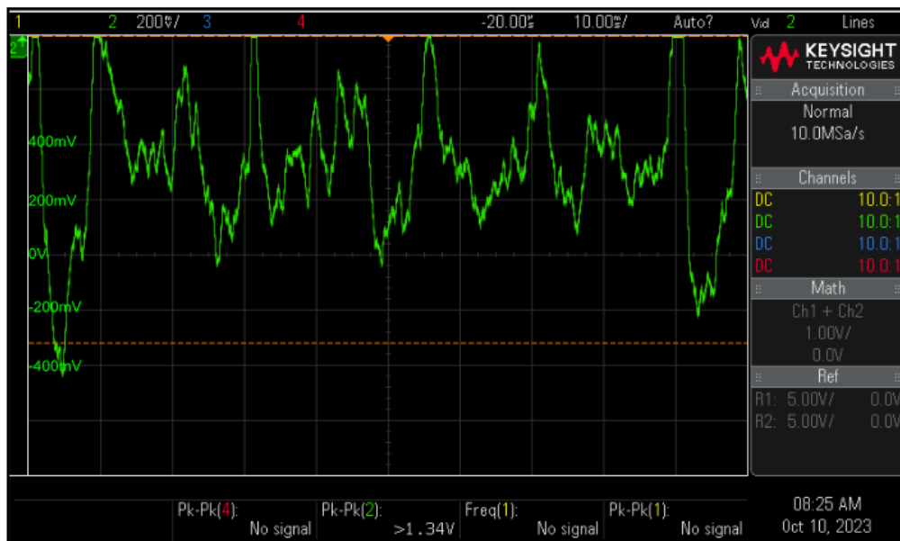
Figure 5-22: Forearm contraction front-end output viewed through an oscilloscope using the same y-axis scale as Figure 5-21.
