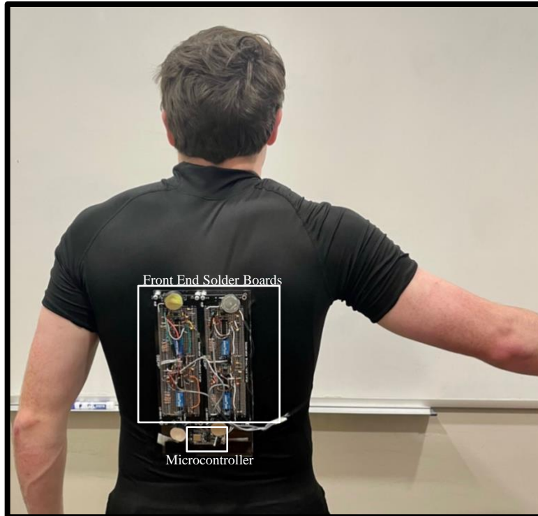
Figure 5: EMG shoulder sleeve in-use on subject.
