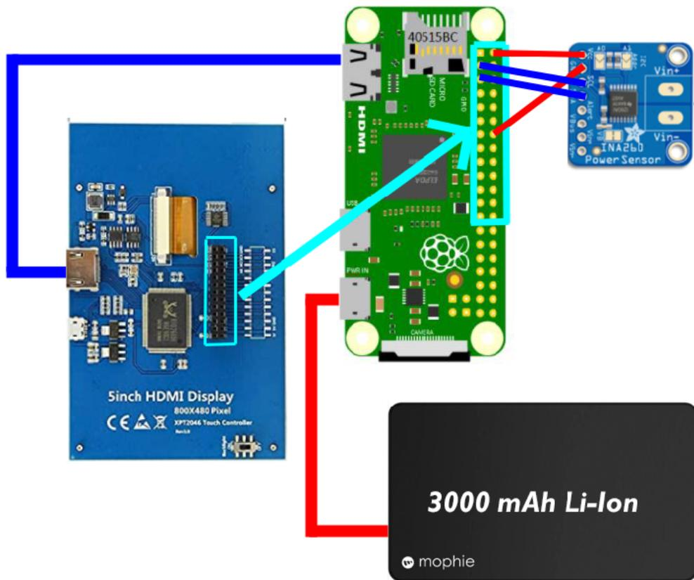
Figure 4: Power Sensor I2C Connections
