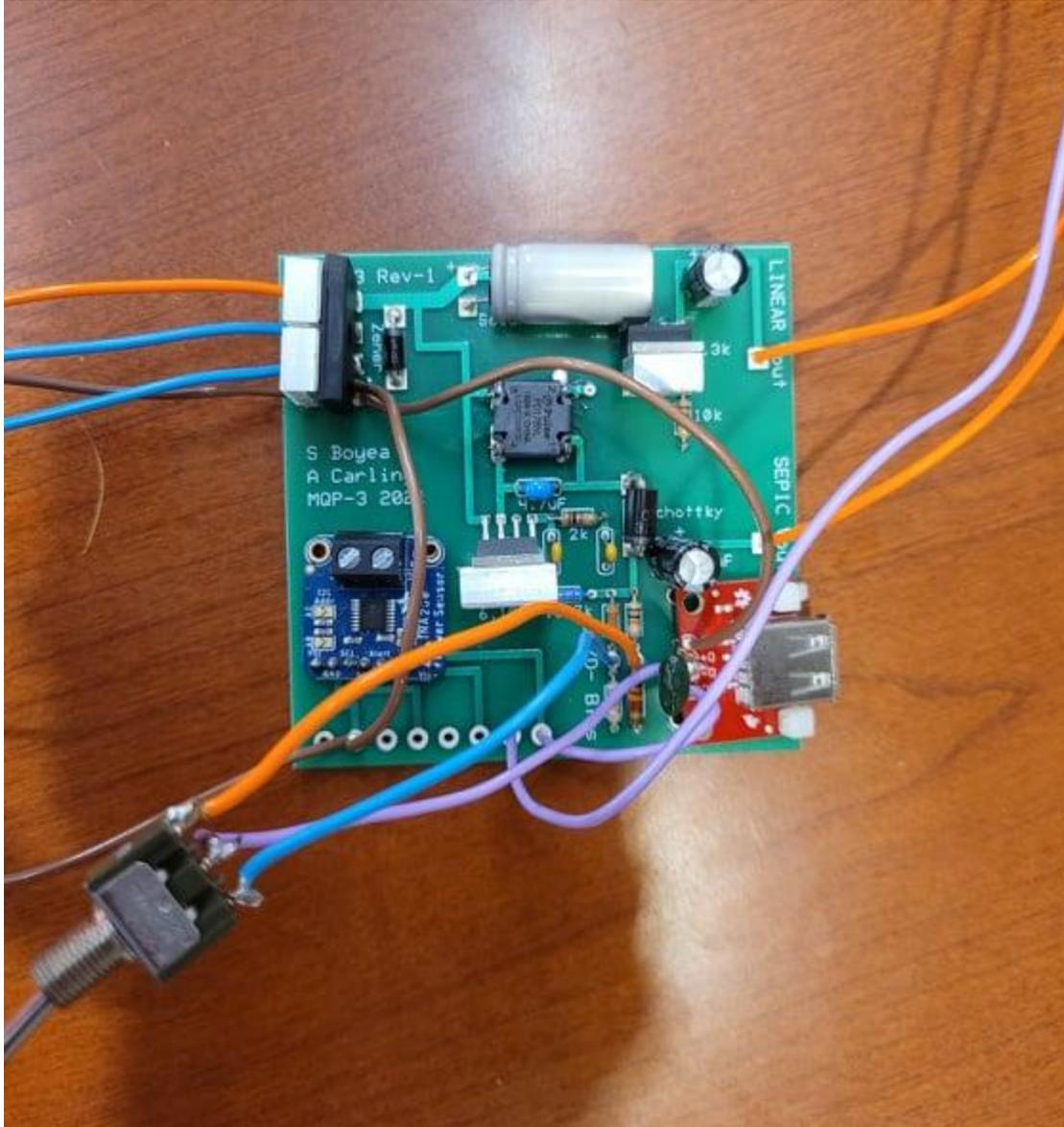
Figure 3: PCB Assembled, Missing Raspberry Pi Connections
