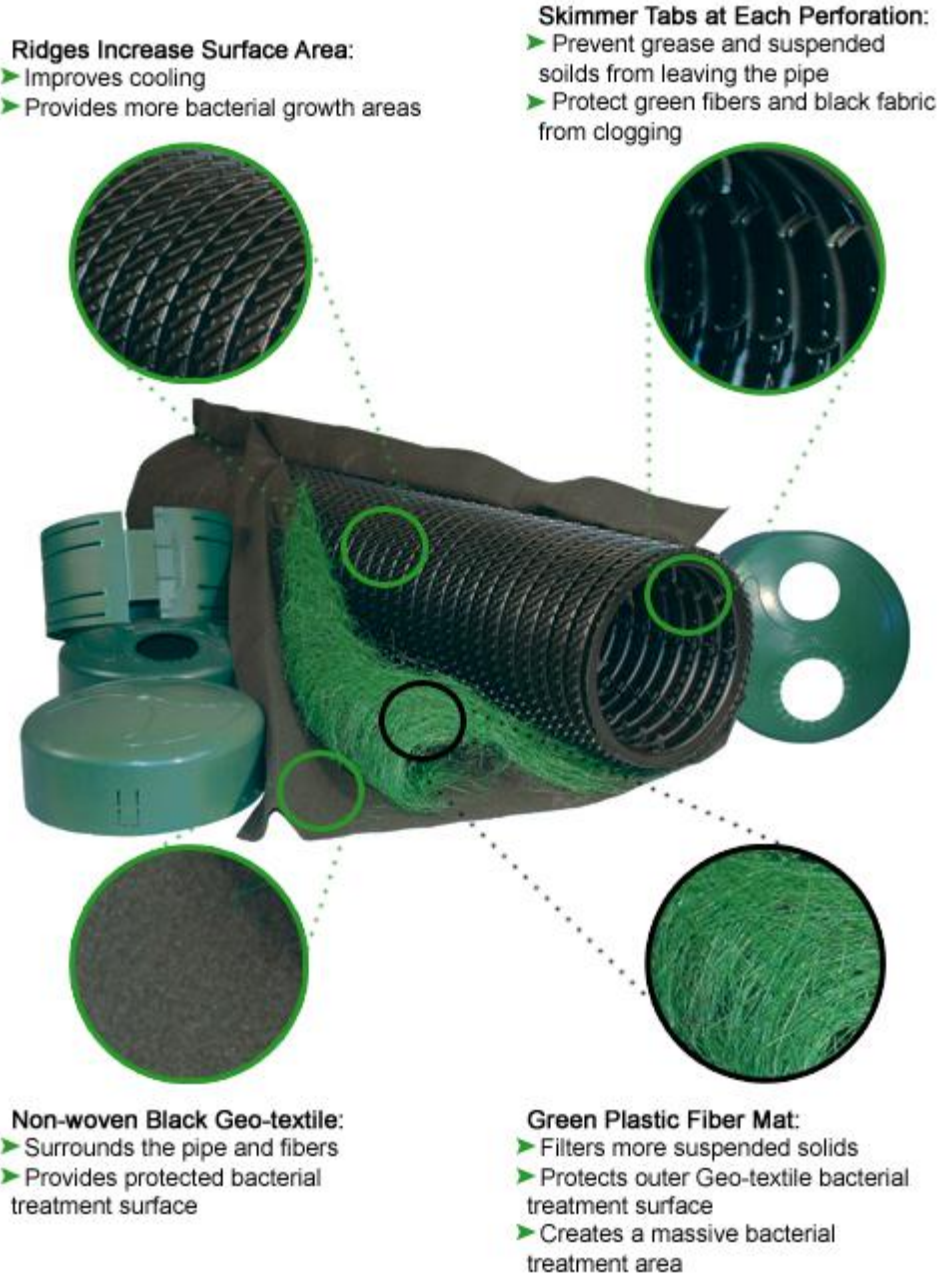
Figure 5: Enviro-Septic Pipe System
