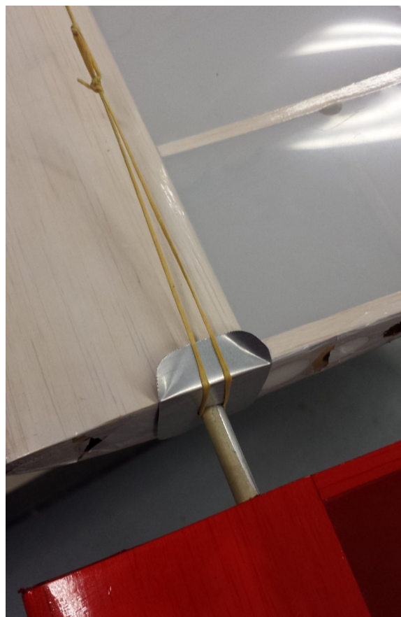
Figure 33-Flying wire wing attachment detail
