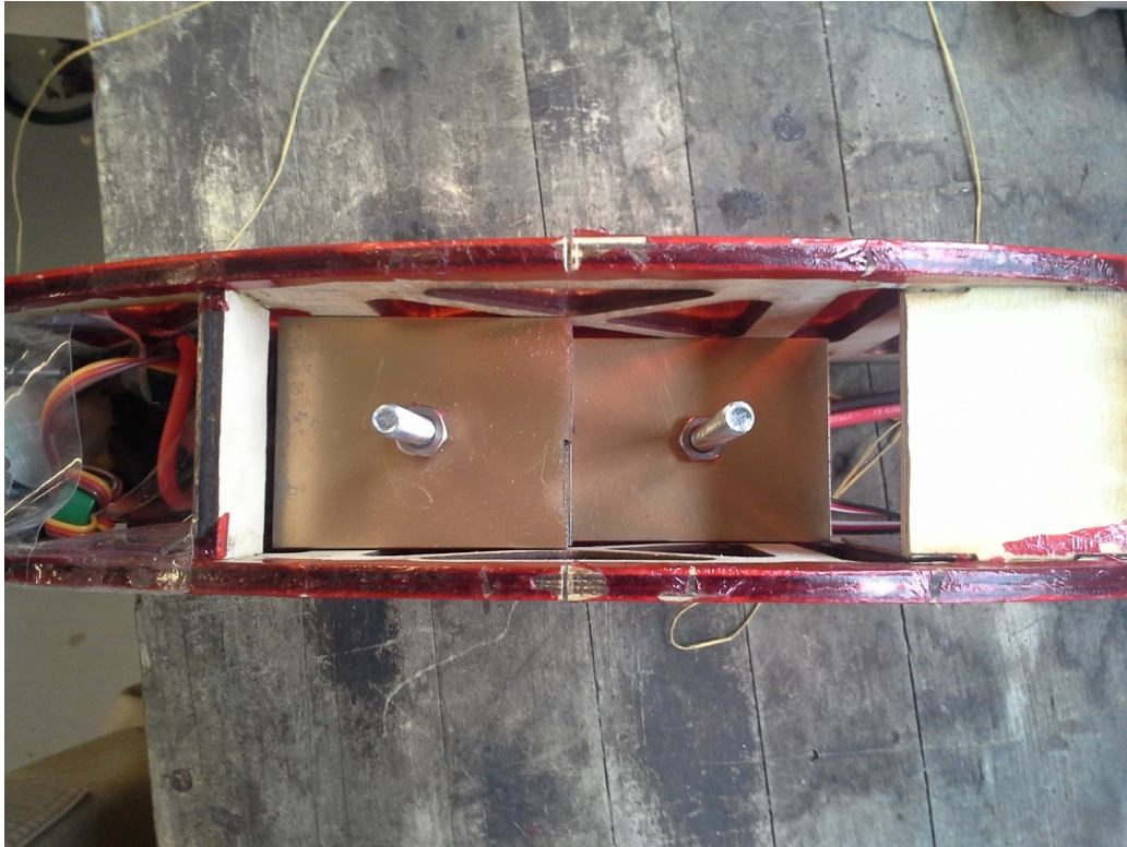
Figure 36-Payload attachment bolts inside the aircraft with a sample payload installed
