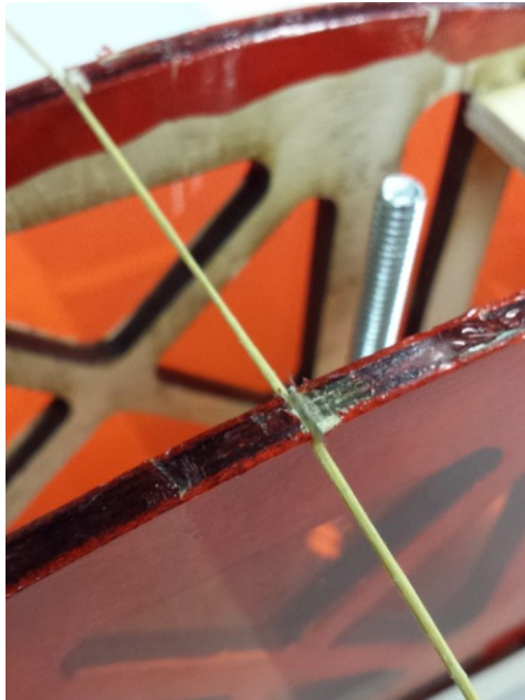
Figure 34-Flying wire fuselage interface
