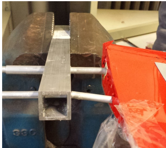
Figure 30-The bent aluminum rod and tube following the failure test
