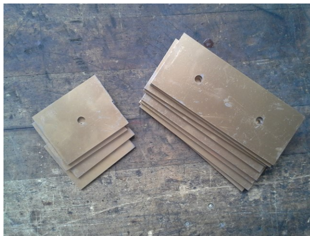
Figure 35-Payload plates. LEFT: Half-sized plates used for CG adjustment. RIGHT: Full payload plates
