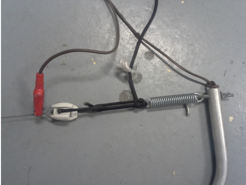
Figure 14-The hot-wire foam cutter and spring modification
