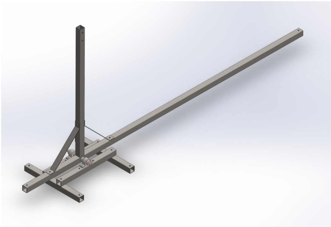
Figure 17-Early SolidWorks model of the thrust stand. It has a 2:1 moment reduction
