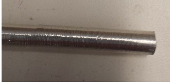
Figure 27-Turned aluminum rod showing the low precision
