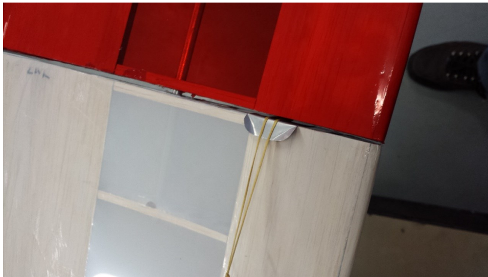
Figure 32-Flying wire wing attachment
