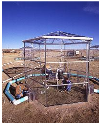
Figure 2.3: Open-top Chamber similar to the ones used for an ITEX experiment. http://www.ars.usda.gov/IS/AR/archive/jul97/gcf0797.htm
