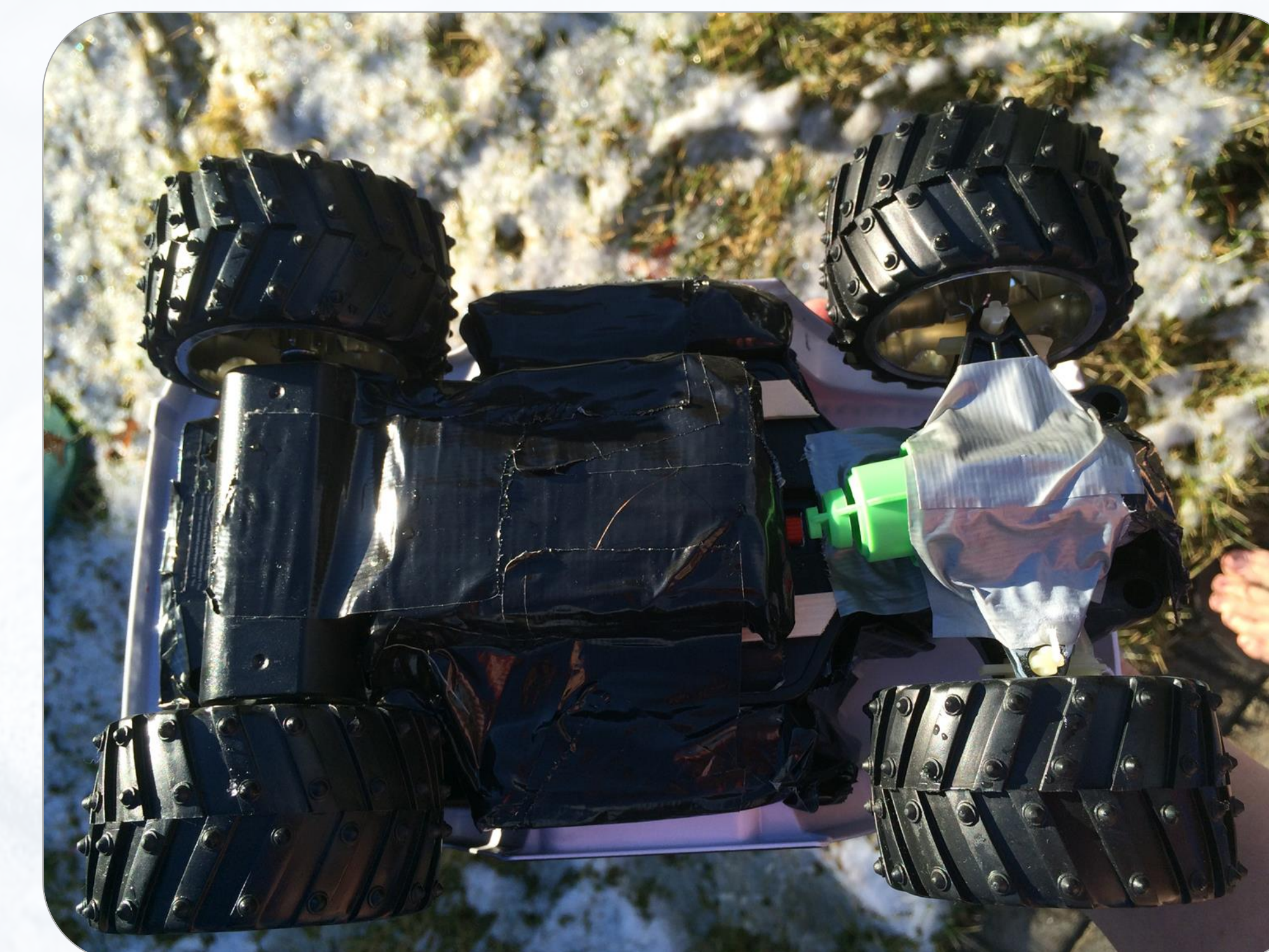
Prototype scale model – waterproofing of underbelly shown here
