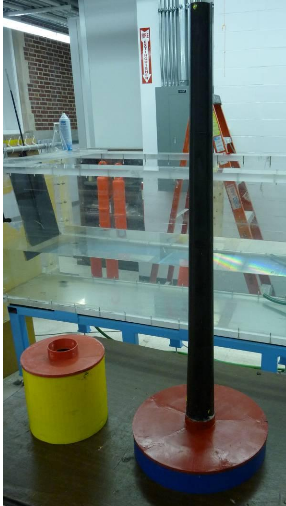
Figure 35. TLP and SDB Tanks with Tower
