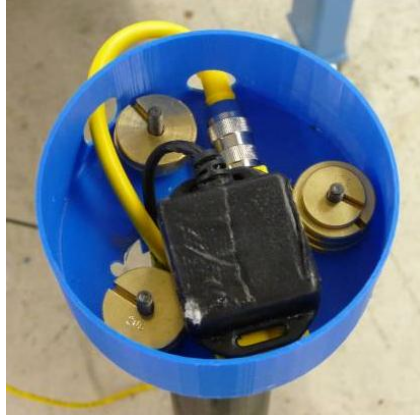
Figure 43. Rotor and nacelle weight with Sensors and Ballast Weights
