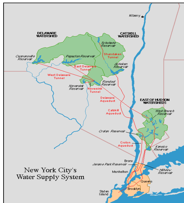
Figure 2: New York City’s Water Supply System (Source: “New York City’s Water Supply System”)
