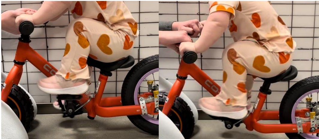
Figure 33: 3" Crank vs Simulated 2" Crank Hip and Knee Locations at Highest Pedal Stroke
