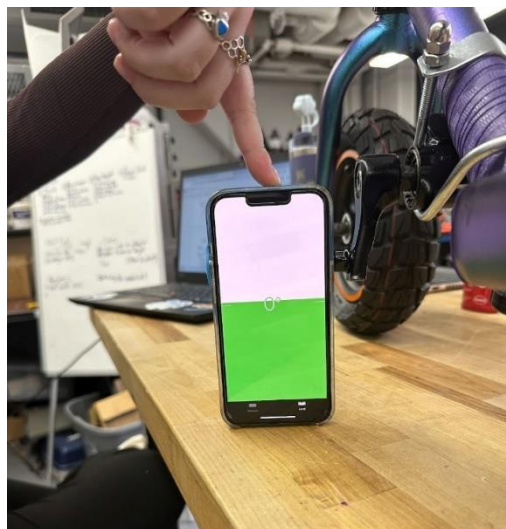
Figure 40: Phone Positioned Parallel to the Pedal with iPhone Measure App
