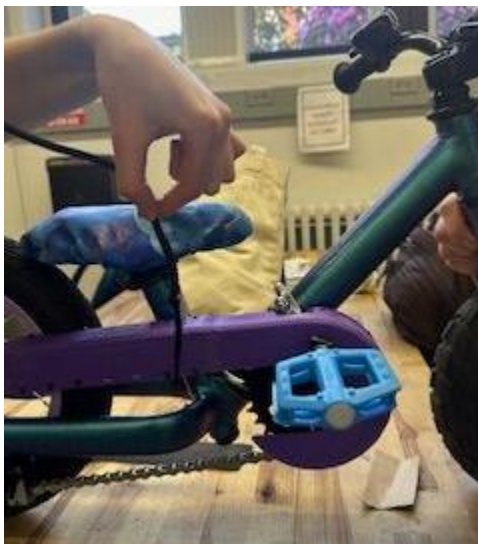
Figure 45: Touch Test Setup with Sweatshirt String
