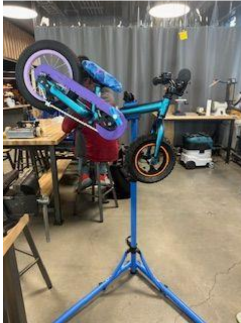
Figure 38: Chain Alignment Test Setup
