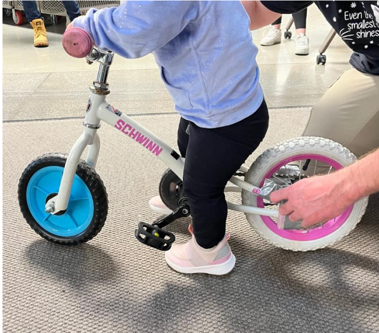
Figure 9: Client's Inseam Equal to the Saddle Height
