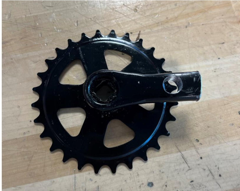
Figure 35: Crank with Gear Cut Down to 2"
