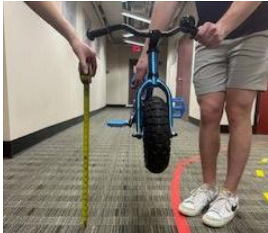
Figure 42: Setup for the Drop Test
