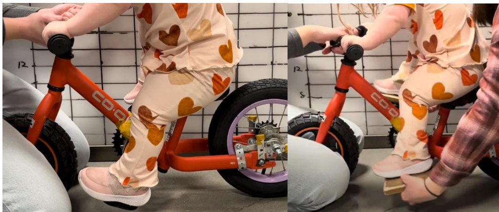
Figure 32: 3" Crank Compared to 2" Crank Position at Lowest Pedal Stroke
