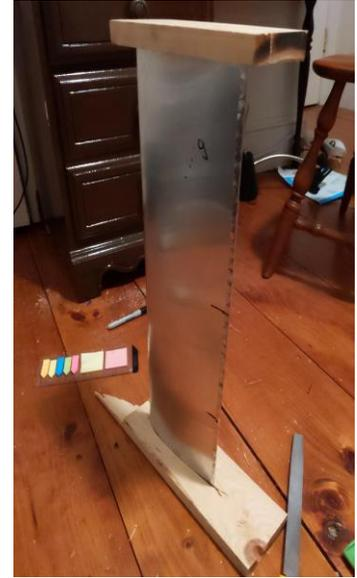
*Figure 12: The framing system used to form the foil to the correct shape while gluing aluminum to wooden support ribs*
