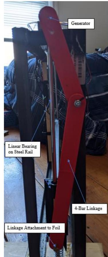
**Figure 24: Fabricated and assembled slider-crank mechanism showing slider rail, 4-bar linkage, and attachment points**
