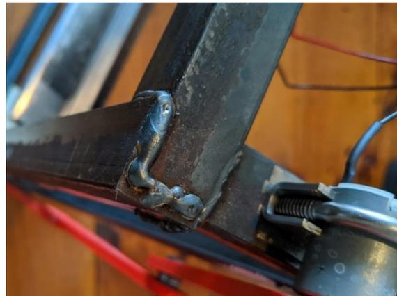
*Figure 22: Example of MIG weld on steel frame*
