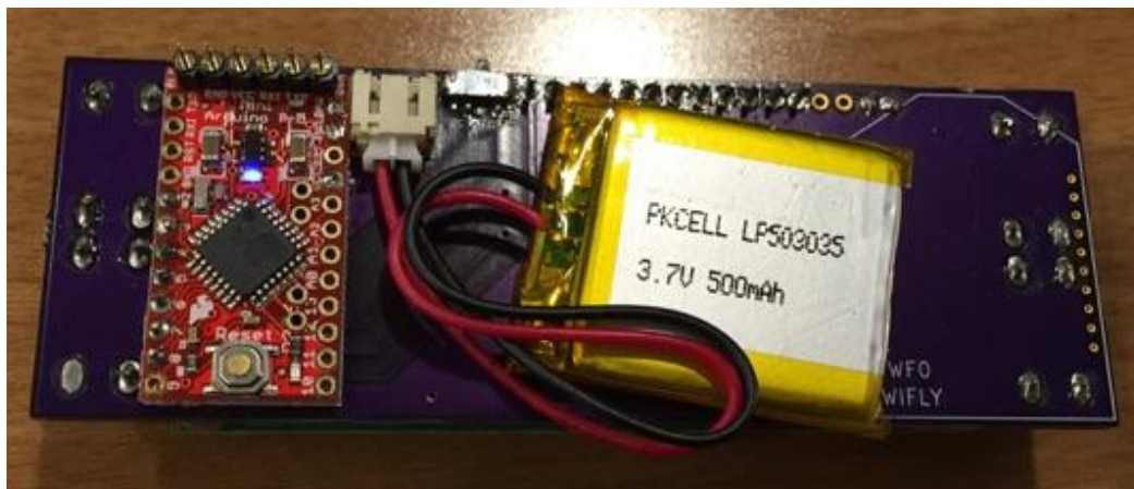
Figure 11: Cyberwatch Prototype 1 backside without housing
